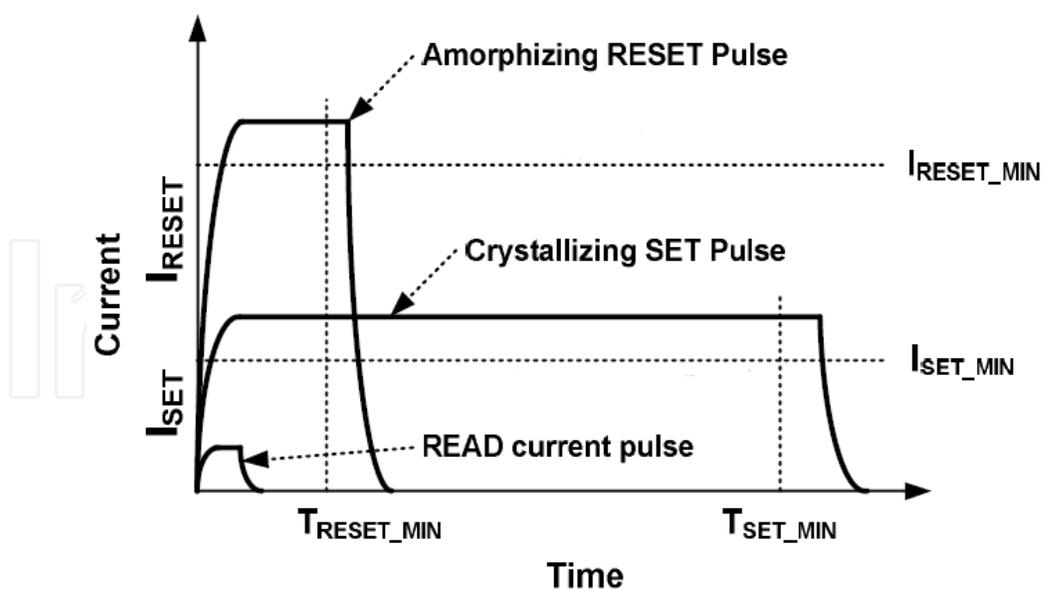
Fig. 5. Current pulses used in reading, SET and RESET processes. [24]
