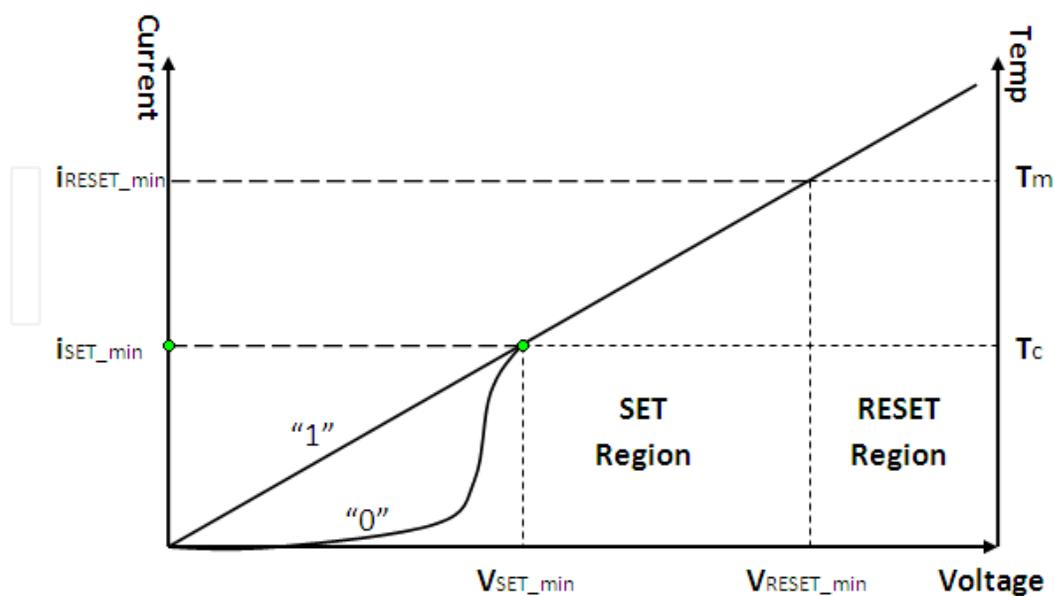
Fig. 3. SET and RESET process of PCM cell. PCM cell temperature is controlled by cell current.  $i_{\text{SET\_min}}$  corresponds to crystallization temperature  $T_c$ ;  $i_{\text{RESET\_min}}$  corresponds to melting temperature  $T_m$ .
