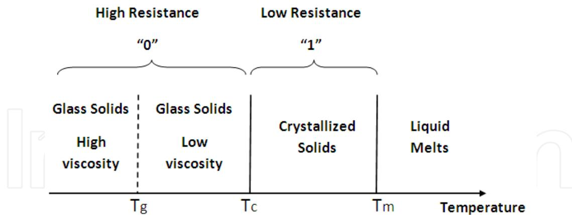
Fig. 1. Phase changes of glassy materials as a function of temperature. Three critical temperatures are observed: glass transition temperature ( $T_g$ ), crystallization temperature ( $T_c$ ) and melting temperature ( $T_m$ ).
