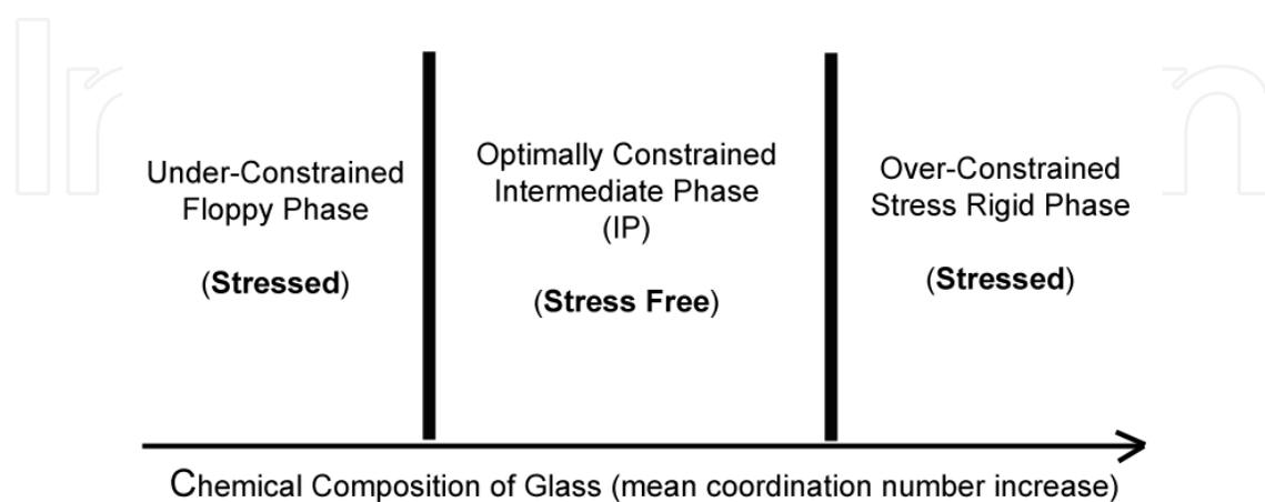
Fig. 2. Elastic phases in chalcogenide glasses as a function of mean coordination number of glasses. Mean coordination number is an indicator of chemical composition.
