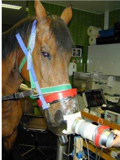
Fig. 6. Intrapleural pressure and air flow measurement in a horse. Intrapleural pressure is measured via an oesophageal balloon connected to a plastic tube. Flow is measured with a Fleisch type pneumotachograph connected to an airtight facemask
