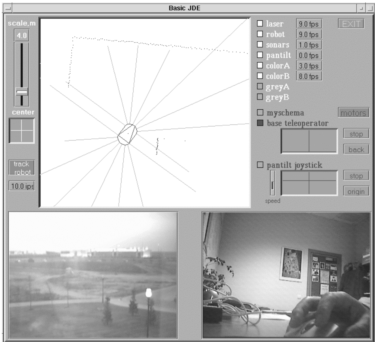
Figure 10. JDE GUI connected to a Pioneer and two different cameras (off-board robot)
