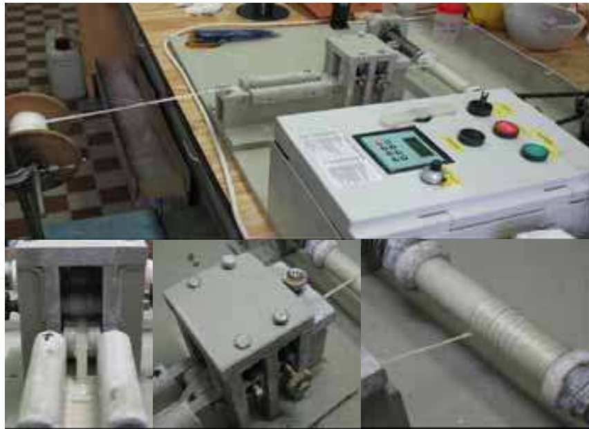
Fig. 1. Details of pultrusion technique used for the preparation of geocomposites
