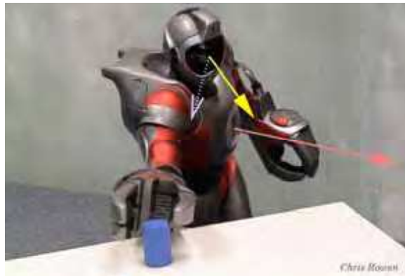
Figure 3. Grasping by a humanoid robot. The object is localized in a visual reference frame (yellow arrow points into gaze direction) by the direction of the dotted, blue arrow. The grasping is performed in a body-centered reference frame (long red arrow). The relation between visual and body-centered systems varies when the head turns
