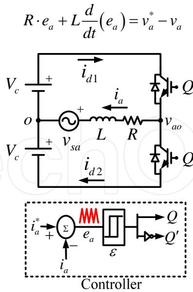
Fig. 1. Single-phase half-bridge inverter with fixed-band hysteresis control.
