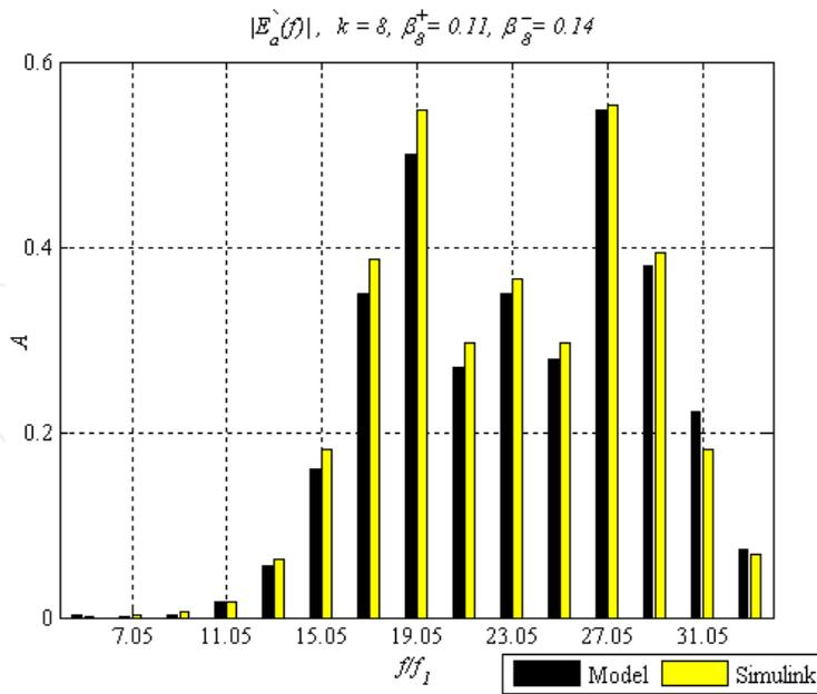
Fig. 18. Error spectrum when the 8<sup>th</sup> dc background distortion exists.
