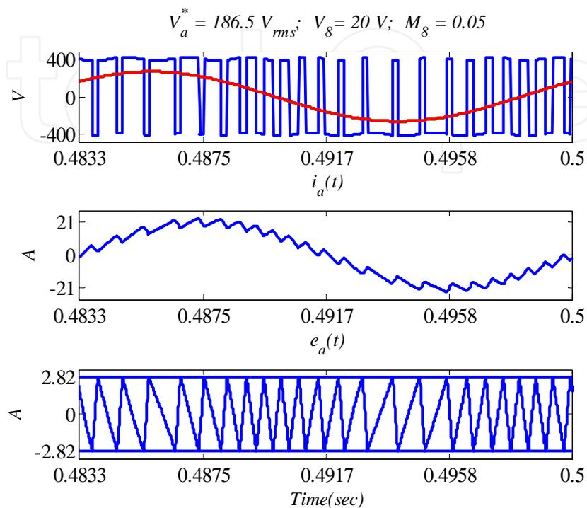
Fig. 16. Effect of injecting the 8<sup>th</sup> dc harmonic voltage on the inverter ac outputs.
