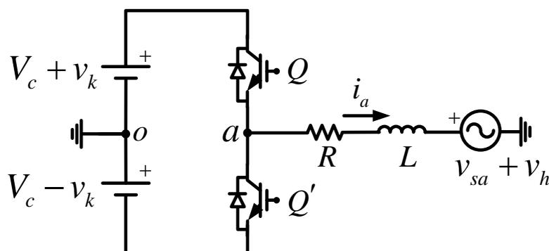
Fig. 7. Hysteresis inverter operating with distorted system voltages.
