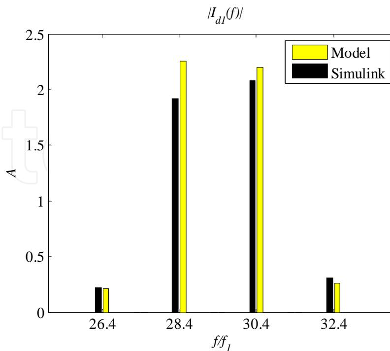
Fig. 24. DC current harmonics under variable-band control.
