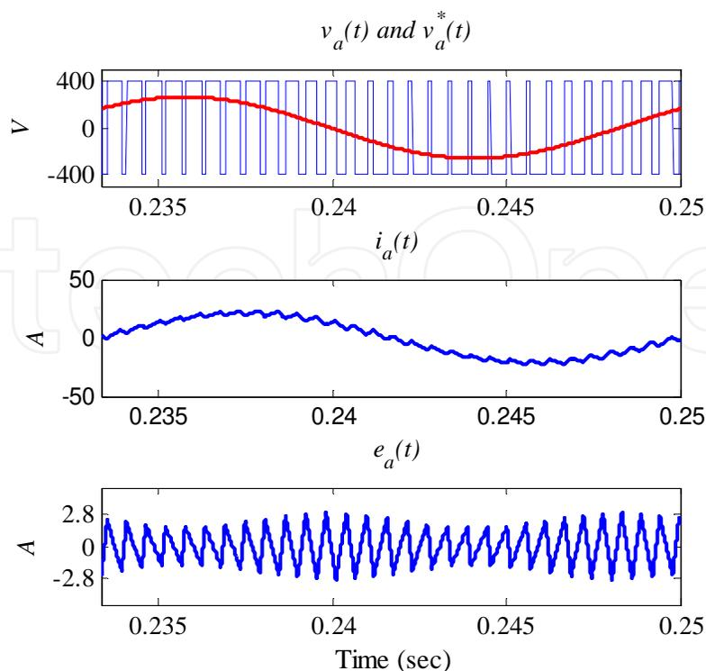
Fig. 19. Instantaneous outputs of the variable-band hysteresis control.
