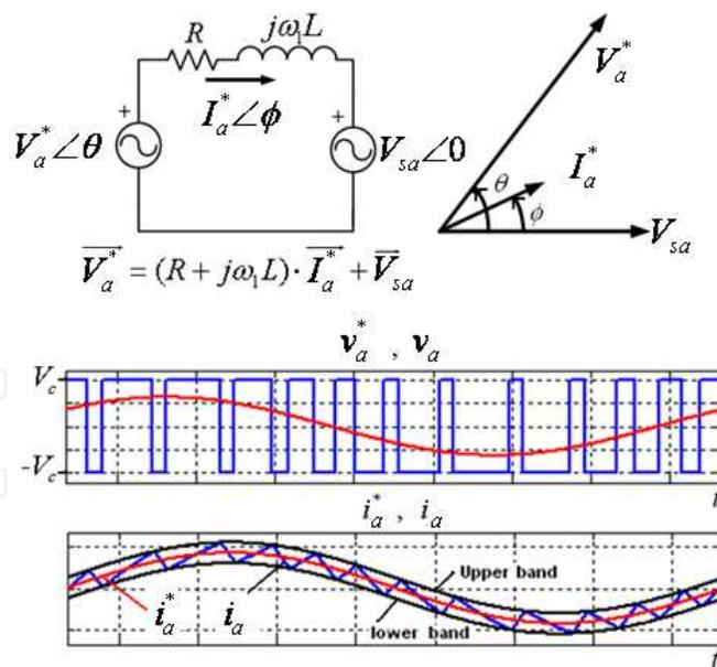
Fig. 2. Reference voltage calculation and the instantaneous outputs.
