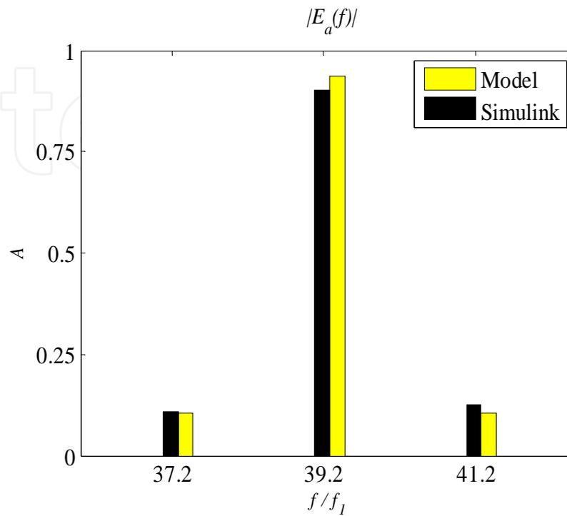
Fig. 23. Inverter harmonic response to 25% reduction in  $L$ .
