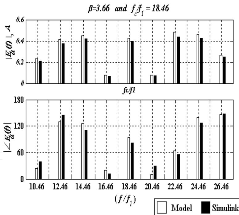
Fig. 10.  $E_a(f)$  when  $V_c$  is decreased to 350V.
