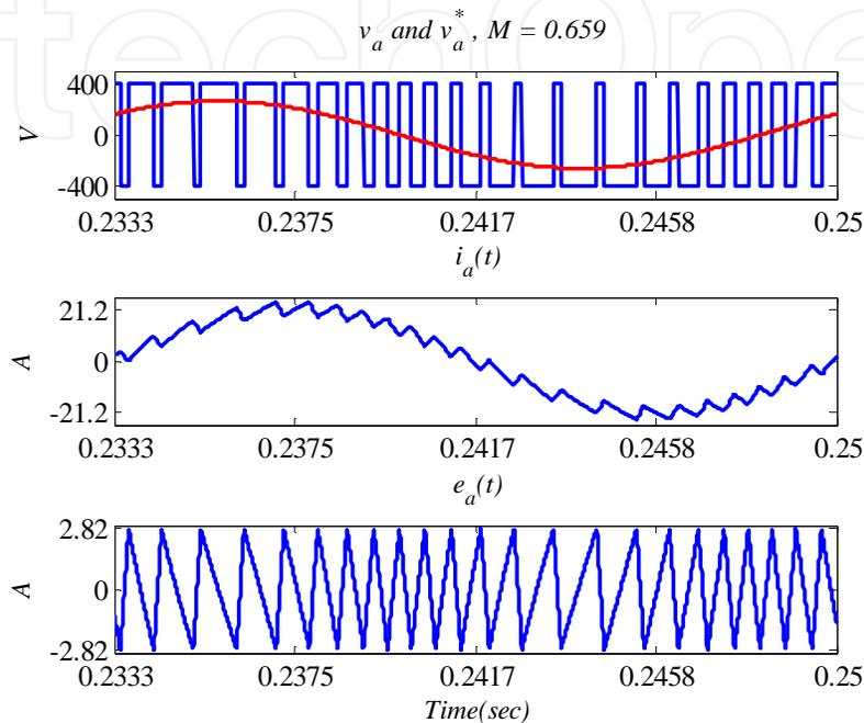
Fig. 8. Inverter ac outputs under fixed-band hysteresis control.
