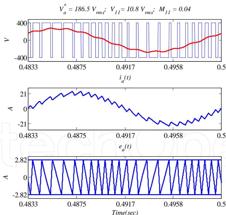
Fig. 13. Effect of injecting the 11<sup>th</sup> ac harmonic voltage on the inverter ac outputs.
