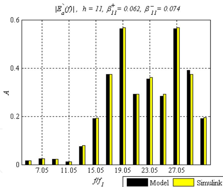
Fig. 15. Error spectrum when  $v_{sa}$  contains the 11<sup>th</sup> oscillator voltage.
