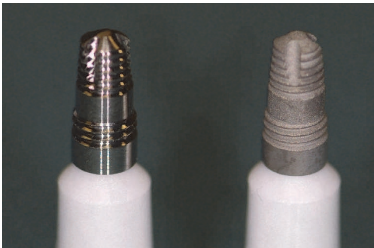
Fig. 3. The machined and nano etched implant surface
