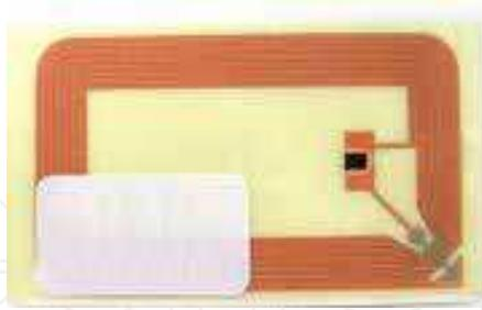
Fig. 1. Example of RFID Card
