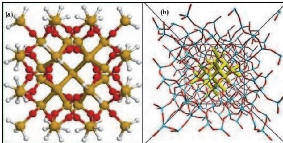
Fig. 7. (a) A stick and ball representation of  $\text{Si}_{17}@\text{Si}_{24}\text{O}_{36}\text{H}_{60}$  (Si clusters embedded in one neutral  $\text{SiO}_2$  shell), (b) The final optimized structure of the  $\text{Si}_{32}$  in  $\beta$ -cristobalite matrix
