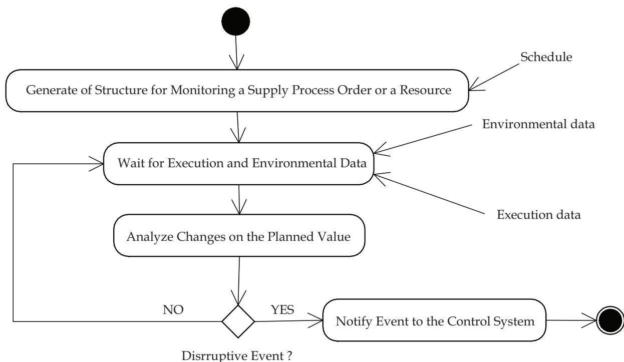
Fig. 6. Functional model of the monitoring subsystem
