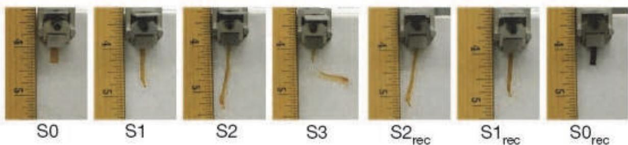
Fig. 5. Quadruple-shape memory properties of PFSA. S0: permanent shape; S1: first temporary shape ( $T_d^1$ : 140 °C); S2: second temporary shape ( $T_d^2$ : 107 °C); S3: third temporary shape ( $T_d^3$ : 68°C); S2<sub>rec</sub>: recovered second temporary shape ( $T_r^1$ : 68°C); S1<sub>rec</sub>: recovered first temporary shape ( $T_r^2$ : 107 °C); S0<sub>rec</sub>: recovered permanent shape ( $T_r^3$ : 140 °C). (Adapted with permission from (Xie, 2010). 2010. Nature Publishing Group Inc.)
