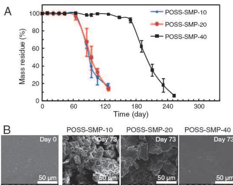
Fig. 8. *In vitro* hydrolytic degradation of POSS-SMPs: (A) %Mass residue of POSS-SMPs in PBS (pH 7.4) as a function of time and PLA arm length. A sample size of 3 was applied. (B) SEM micrographs of POSS-SMPs before and after 73-day incubation in PBS at 37 °C. (Adapted with permission from (Xu & Song, 2010). 2010, the National Academy of Sciences, USA.)
