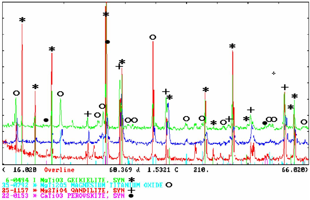
Fig. 9. XRD pattern of plasma sprayed MCT
