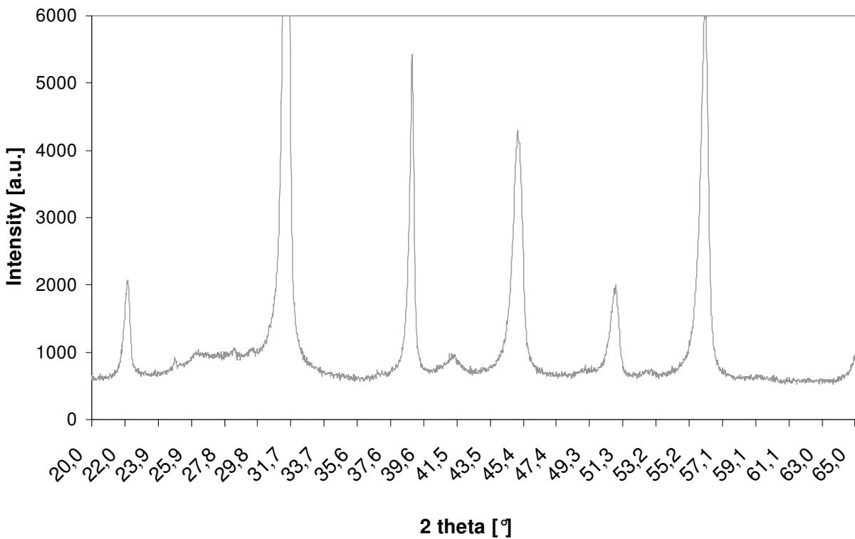
Fig. 10. XRD pattern of plasma sprayed BT coating
