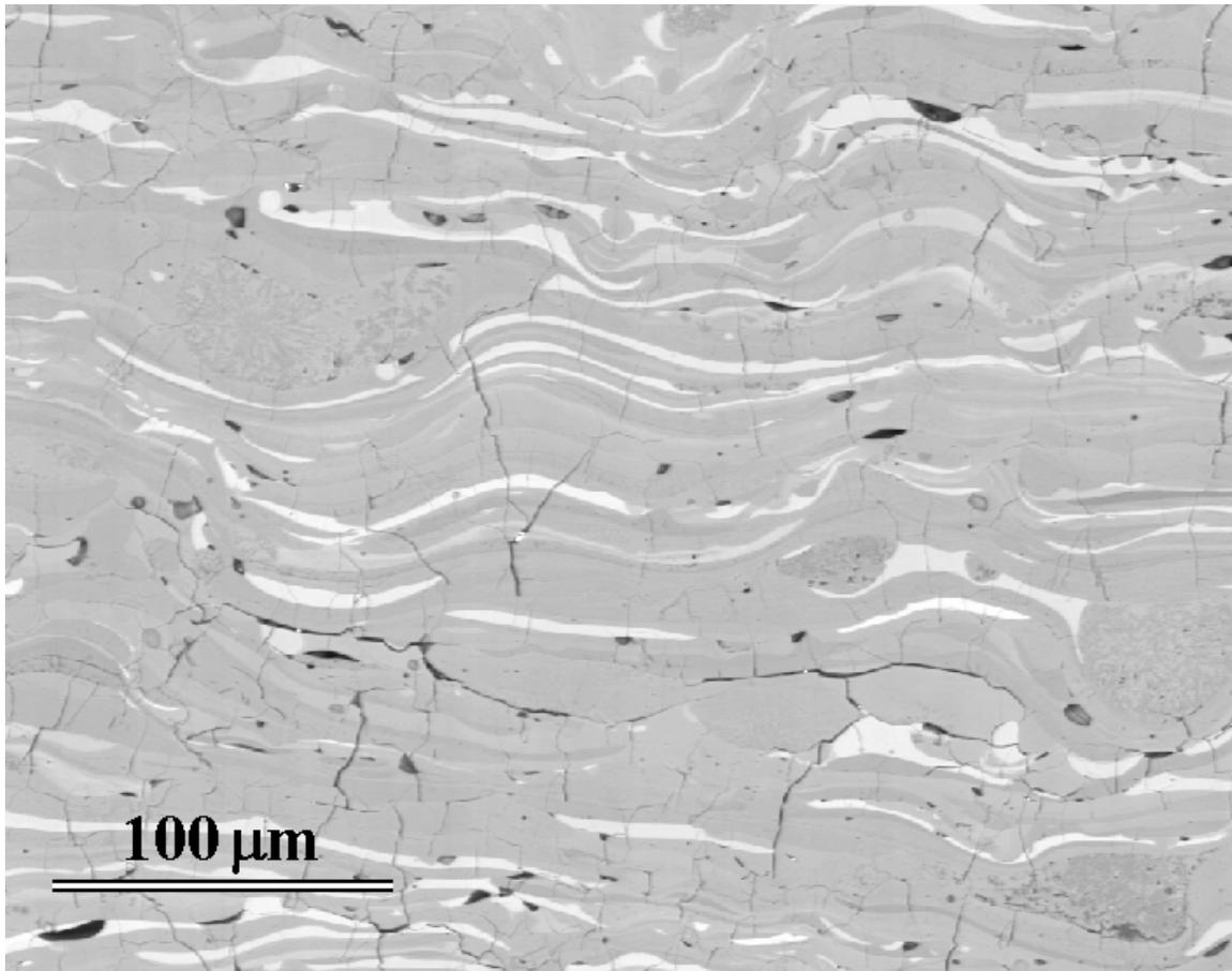
Fig. 5. SEM-BE image showing the lamellar microstructure
