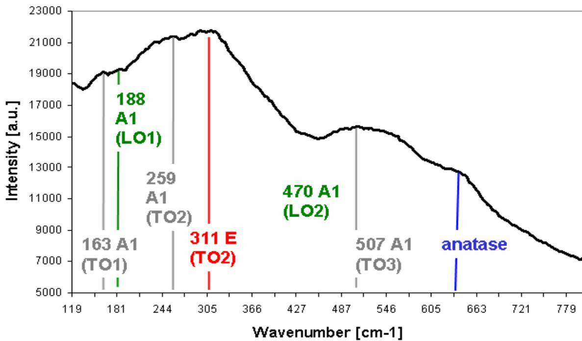
Fig. 6. Raman spectrum of plasma sprayed BaTiO<sub>3</sub>
