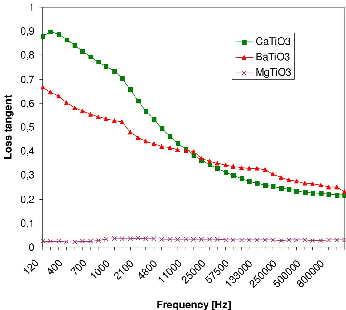
Fig. 15. Frequency dependence of the loss tangent of plasma sprayed BaTiO<sub>3</sub>, CaTiO<sub>3</sub>, and MgTiO<sub>3</sub> at room temperature
