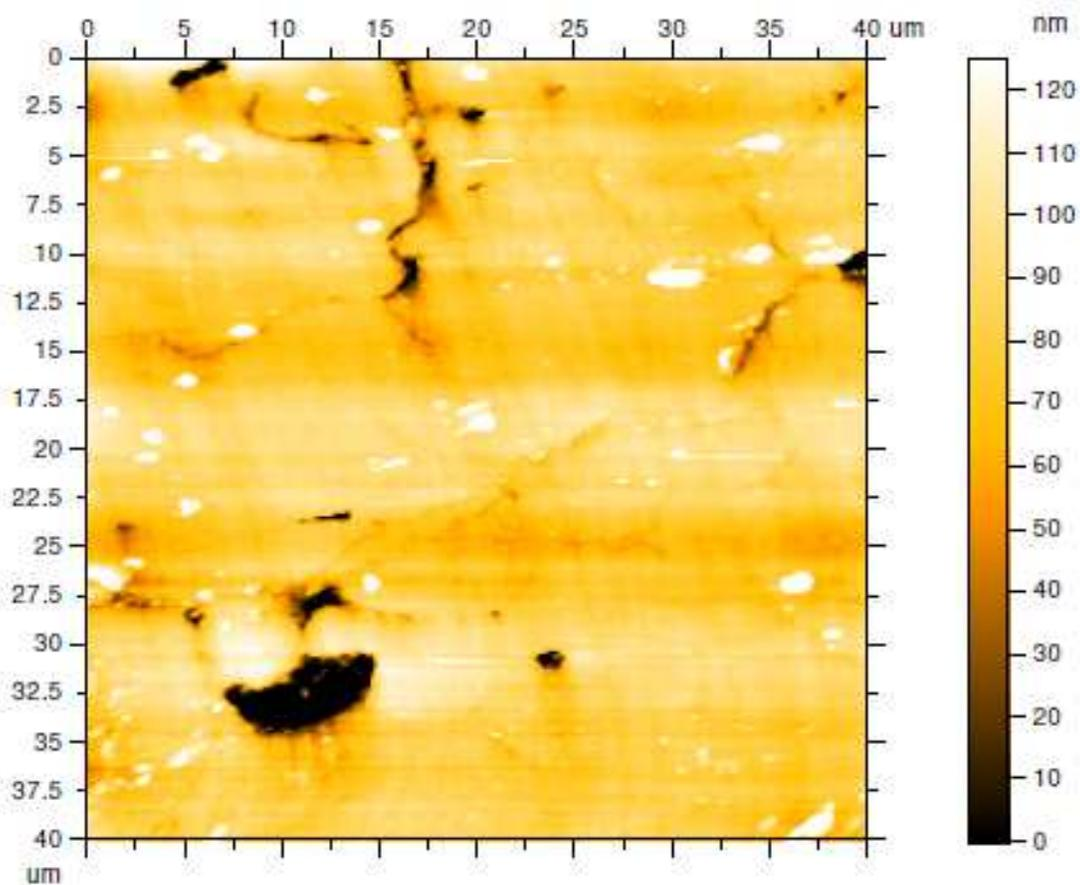
Fig. 17. AFM contact mode image of BaTiO<sub>3</sub> (in plane orientation). Roughness representation: peaks are lighter and valleys darker (black color represents pores)
