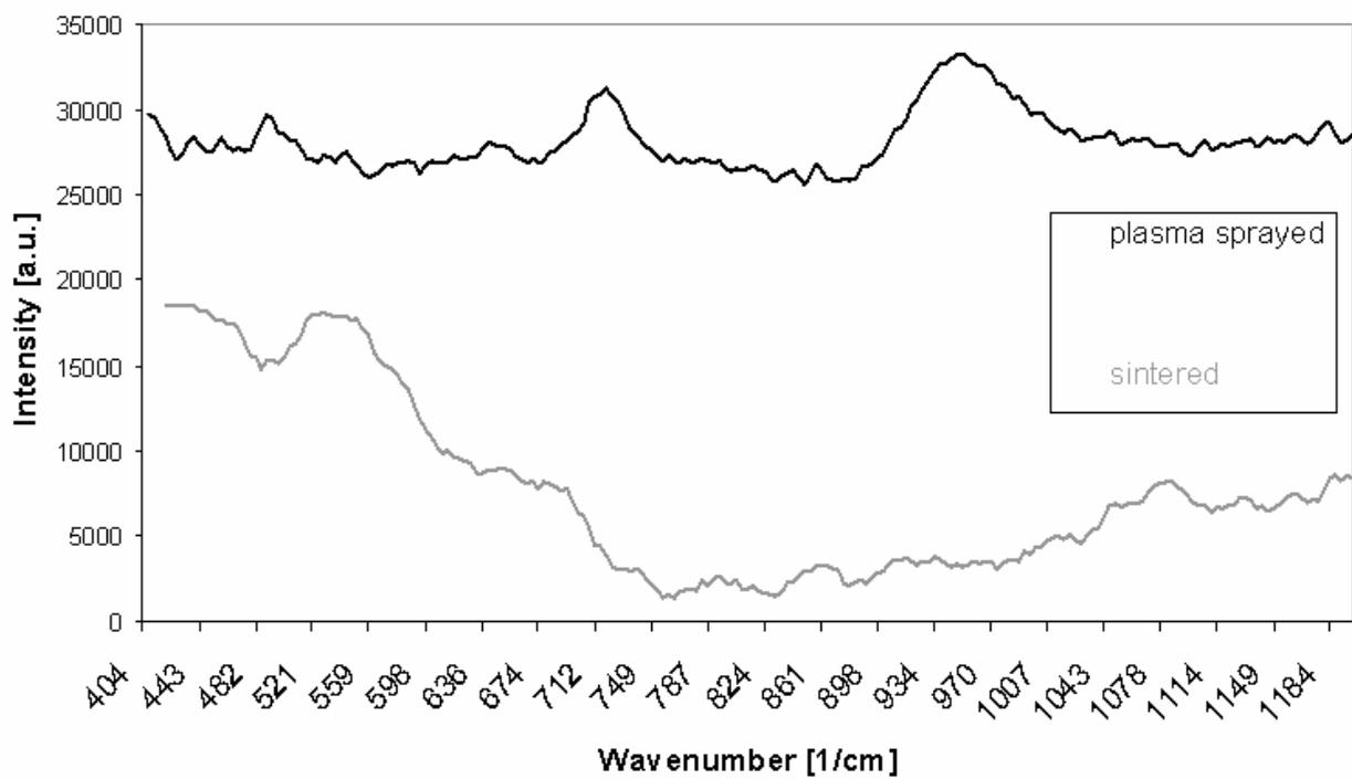
Fig. 2. Raman spectrum of MgTiO<sub>3</sub>
