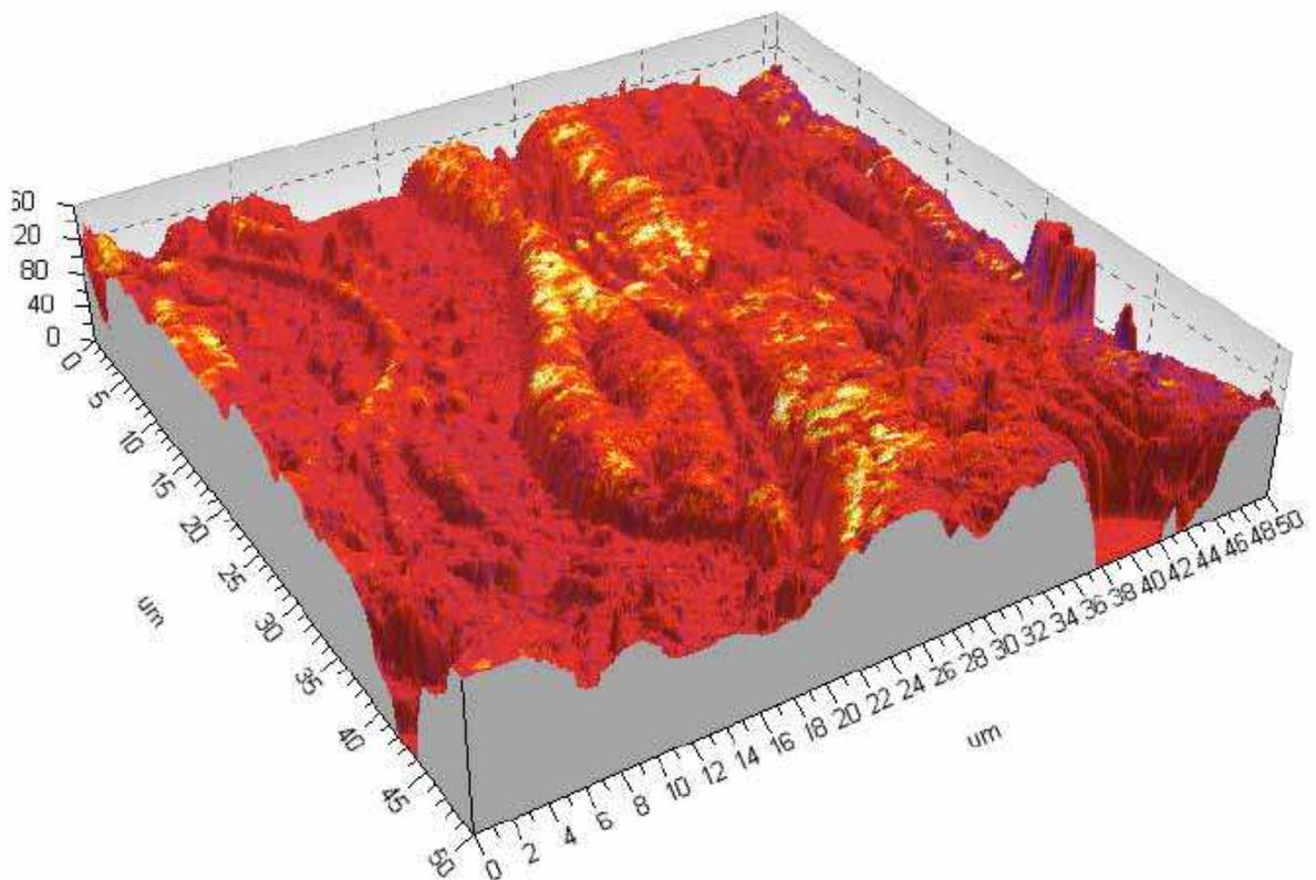
Fig. 20. Superposition of the AFM contact mode image and SMM image - BaTiO<sub>3</sub> cross section. Hard and high-permittivity Ti-rich lamellas are yellow
