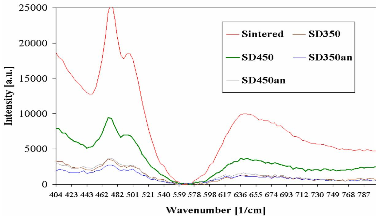
Fig. 1. Raman spectrum of CaTiO<sub>3</sub>
