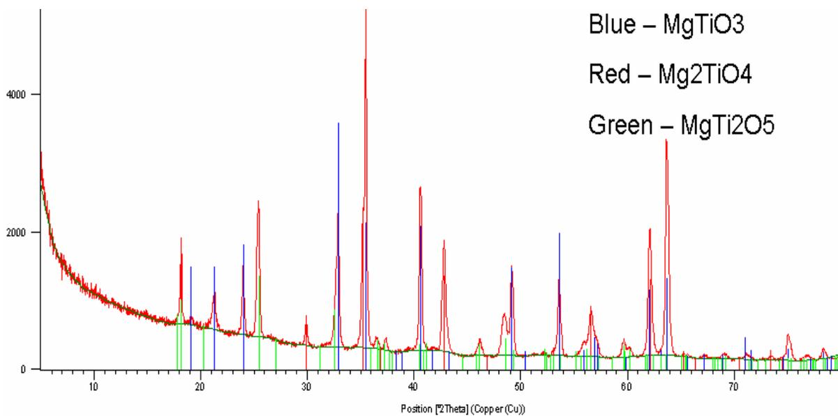
Fig. 8. XRD pattern of plasma sprayed  $\text{MgTiO}_3$
