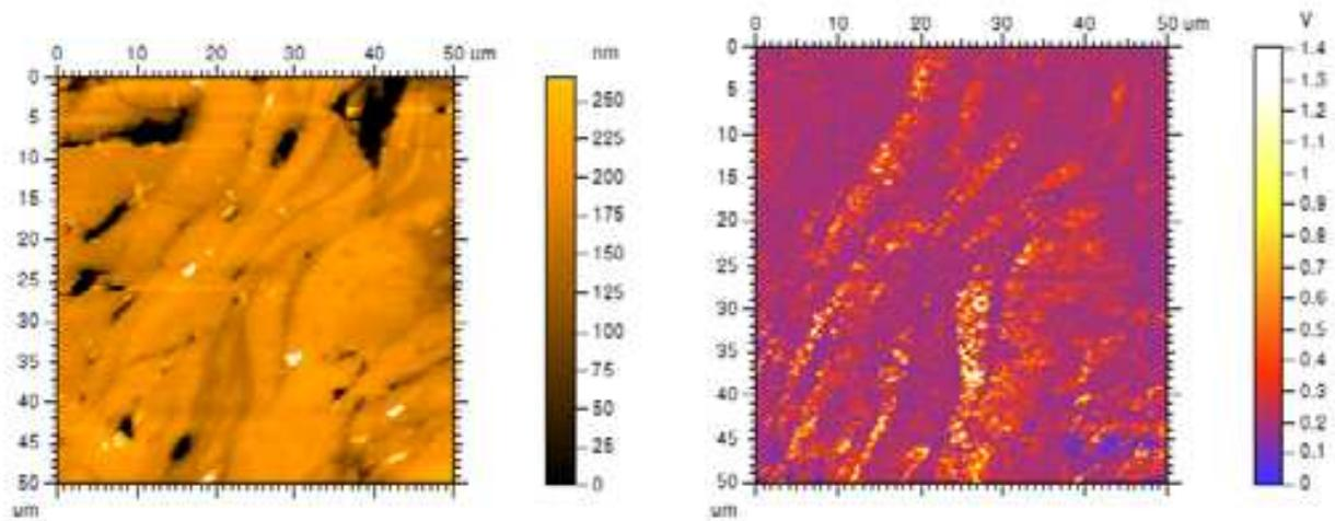
Fig. 19. AFM contact mode image of BaTiO<sub>3</sub> (cross sectional orientation). Left: Roughness representation: peaks are lighter and valleys darker (black color represents pores). Right: Scanning microwave microscopy image of BaTiO<sub>3</sub> (cross sectional orientation) - artificially colored: blue and red zones represent different relative permittivity
