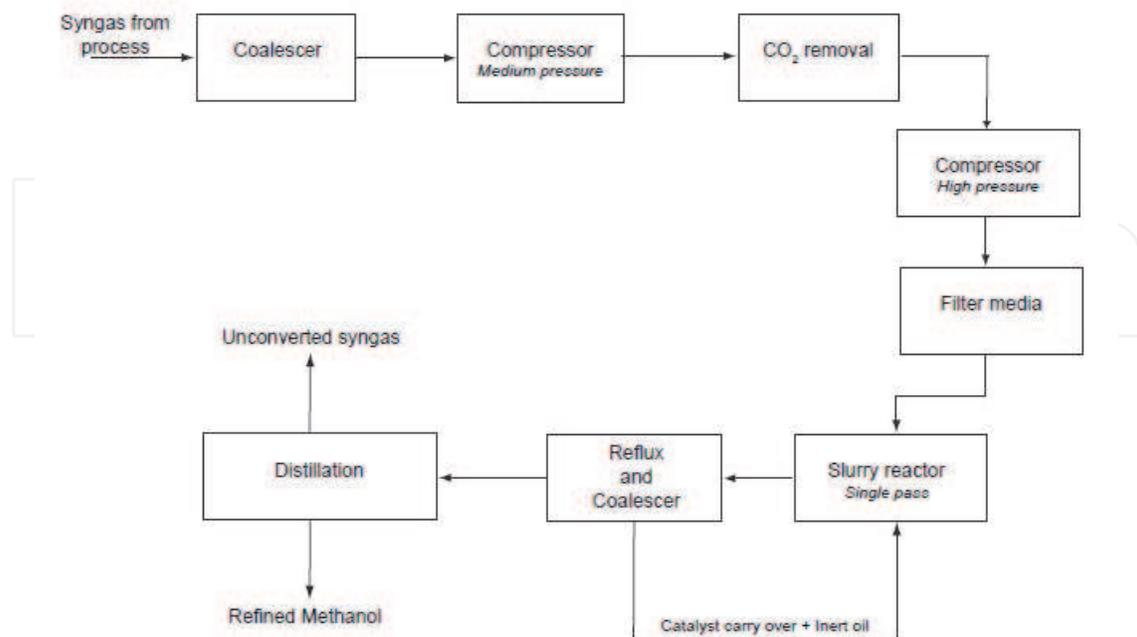
Fig. 5. Enkern Inc. liquid phase methanol process
