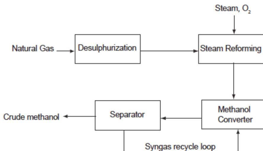
Fig. 4. Haldor Topsoe methanol synthesis process (Sunggyu, 2007).
