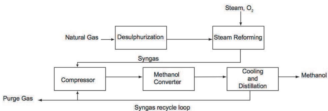
Fig. 3. Simplified Methanol Synthesis PFD (Spath and Dayton, 2003).
