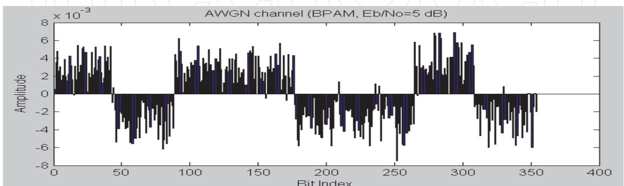
Fig. 4.9. AWGN channel output (BPAM), where  $E_b/N_0=5$  dB.
