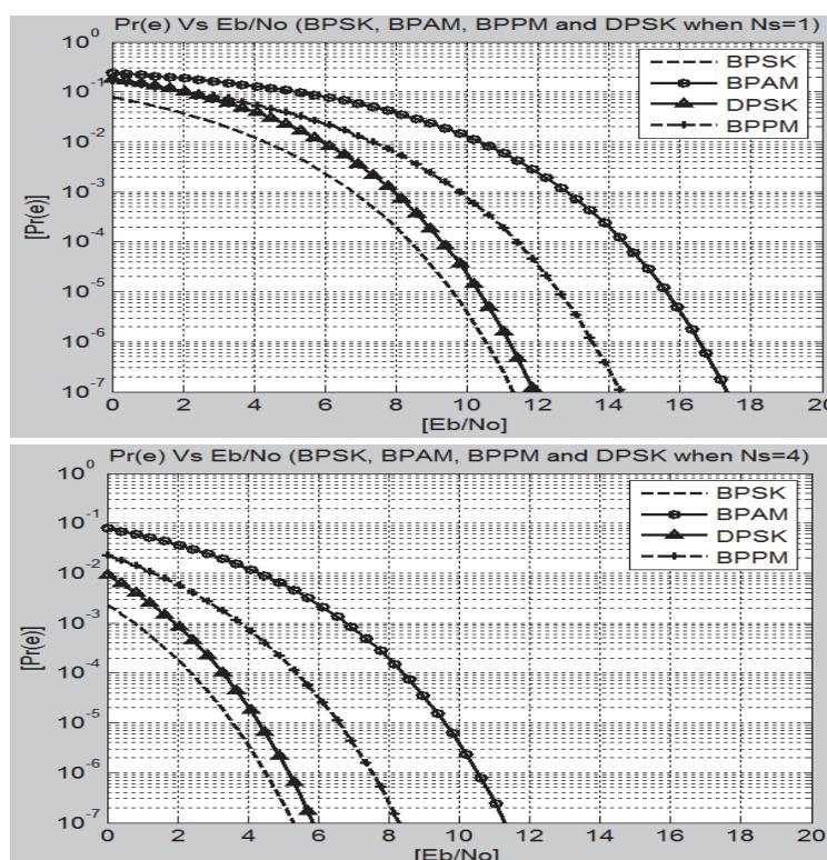
Fig. 4.10. BER performance BPSK, BPAM, DPSK, BPPM ( $N_s=1, 4$ ).
