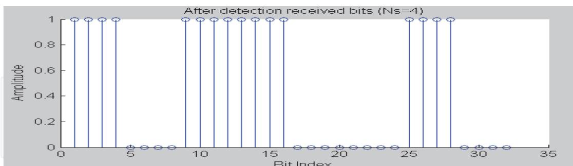
Fig. 4.15. Output after detection (10110010),  $N_s = 4$ .
