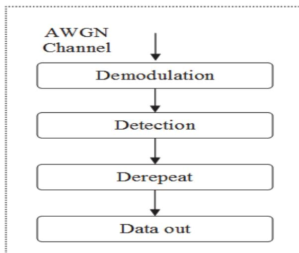
Fig. 4.3. DS-UWB energy detection receiver.
