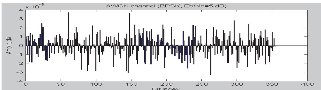
Fig. 4.8. AWGN channel output (BPSK), where  $E_b/N_0=5$  dB.
