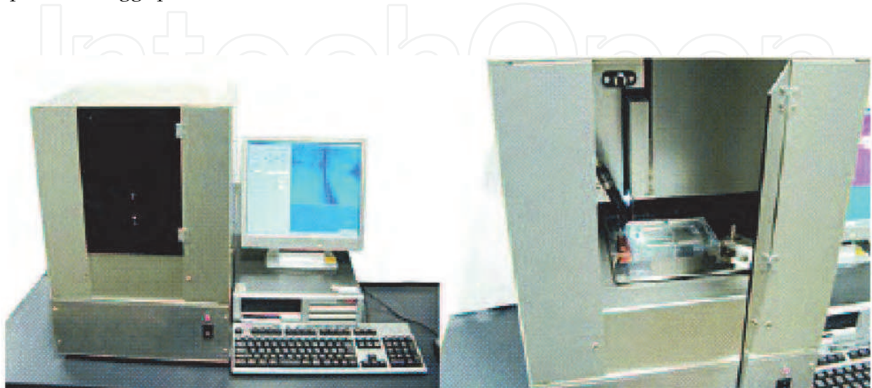
Fig. 2. Fully automated injection system for zebrafish
