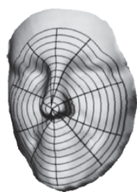
Fig. 6. Geodesic paths and circles defined over a face surface. The tip of the nose was selected as the geodesic pole (Mpiperis et al., 2007)
