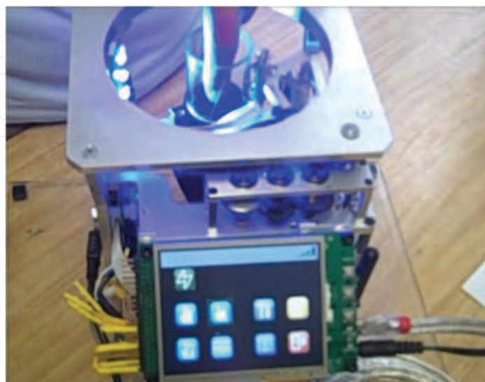
Fig. 5. Front view of the contactless line scans fingerprinting system
