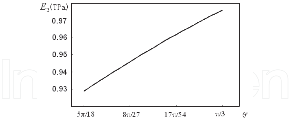
Fig. 13. Elastic modulus of the equivalent model of graphene at perpendicular direction to the 0° fiber
