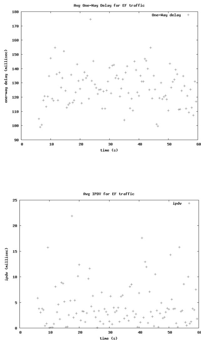
Fig. 2. One Way Delay (OWD) and Jitter (IPDV) for DiffServ only
