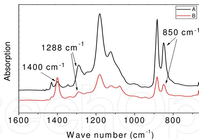
Fig. 5. FT-IR analysis of the  $\beta$  phase of P(VDF-TrFE) polymer films (A and B) with different polymer chain alignment characteristics. In sample A, the polymer chains are aligned parallel to the substrate, and in sample B, the polymer chains are tilted and some portions are aligned perpendicular to the substrate.
