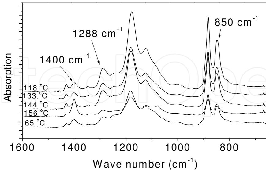
Fig. 16. Polarized FT-IR results for P(VDF-TrFE) films annealed at different temperatures. The different absorption at 850, 1288 and 1400 cm<sup>-1</sup> bands represent the annealing temperature affects on polymer chain alignment. Reprinted from [Mao et al., 2010a] with permission.
