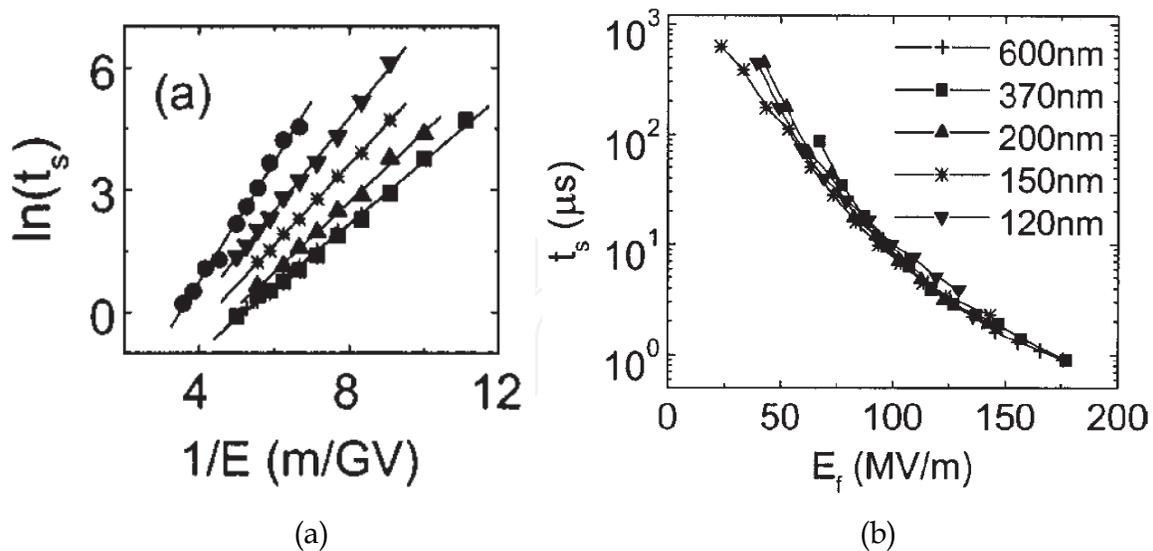
Fig. 18. (a) Switching time as a function of  $1/E$  with different film thicknesses for (from right to left) 600, 370, 200, 150, 120 nm films and (b) switching time as a function of  $E_f$  using the interfacial layer model. Reprinted from [Xia et al., 2001] with permission.
