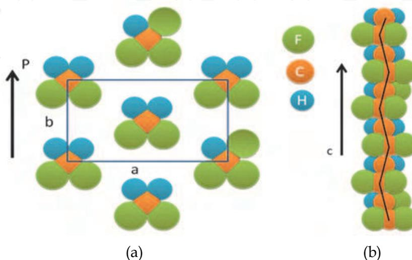
Fig. 2. (a) The schematic of the  $\beta$  phase crystal structure for P(VDF-TrFE) copolymer in the ab plane (the c axis is normal to the ab plane), and (b) along the c axis of the all-trans (TTTT) zigzag planar configuration from the top view.
