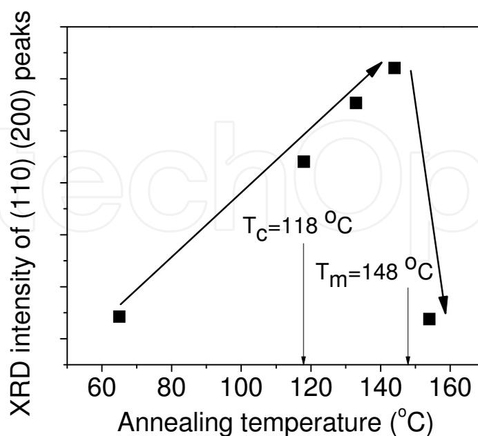
Fig. 15. XRD intensity of (110), (200) orientations after different annealing temperatures. The (110), (200) diffraction peaks at  $2\theta=19.9^\circ$  are attributed to the  $\beta$  phase of P(VDF-TrFE).
