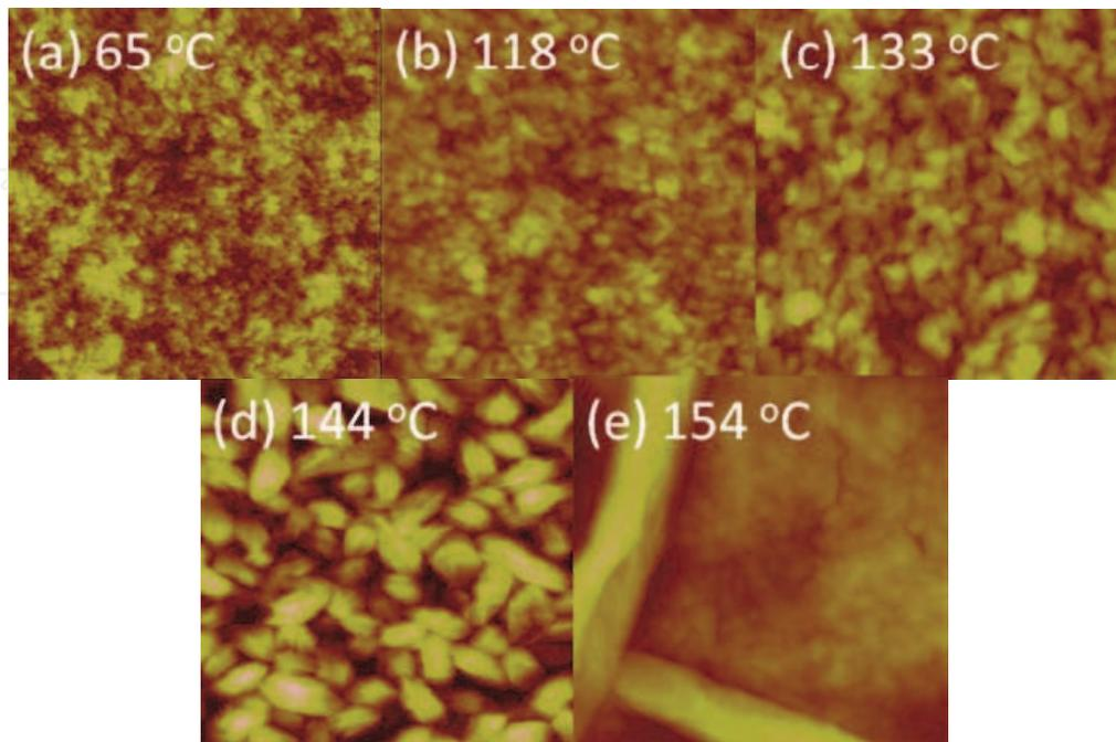
Fig. 14. AFM  $1\mu\text{m}\times 1\mu\text{m}$  height images of P(VDF-TrFE) film annealed at different temperatures. (a) 65 °C, (b) 118 °C, (c) 133 °C, (d) 144 °C, and (e) 154 °C. The height scales are 30 nm for (b), (c), (d), 10 nm for (a), and 100 nm for (e). All of the images were collected at room temperature.
