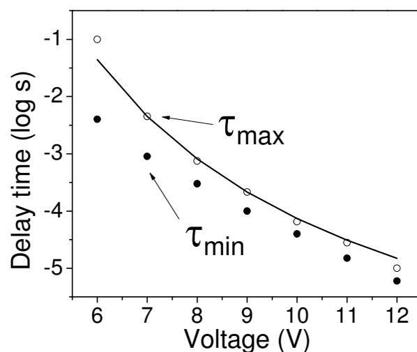
Fig. 12. Experimental  $\tau_{\max}$  and  $\tau_{\min}$  data from Figure 11 plotted as a function of applied voltage, and the fitting for  $\tau_{\max}$  in positive polarization region. Reprinted from [Mao et al, 2010b] with permission.
