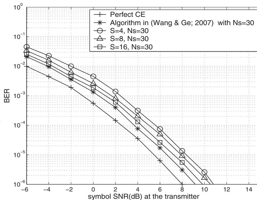
Fig. 6. BER performance of Perfect CE, the algorithm proposed in (Wang & Ge, 2007) and the proposed algorithm with different number of templates ( $S = 4, 8, 16$ ), when the length of the training sequence  $N_s$  is 30.
