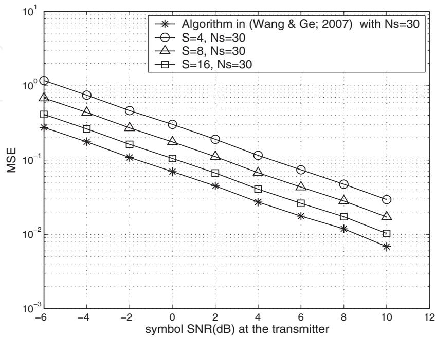
Fig. 5. MSE performance of the algorithm proposed in (Wang & Ge, 2007) and the proposed algorithm with different number of templates ( $S = 4, 8, 16$ ), when the length of the training sequence  $N_s$  is 30.
