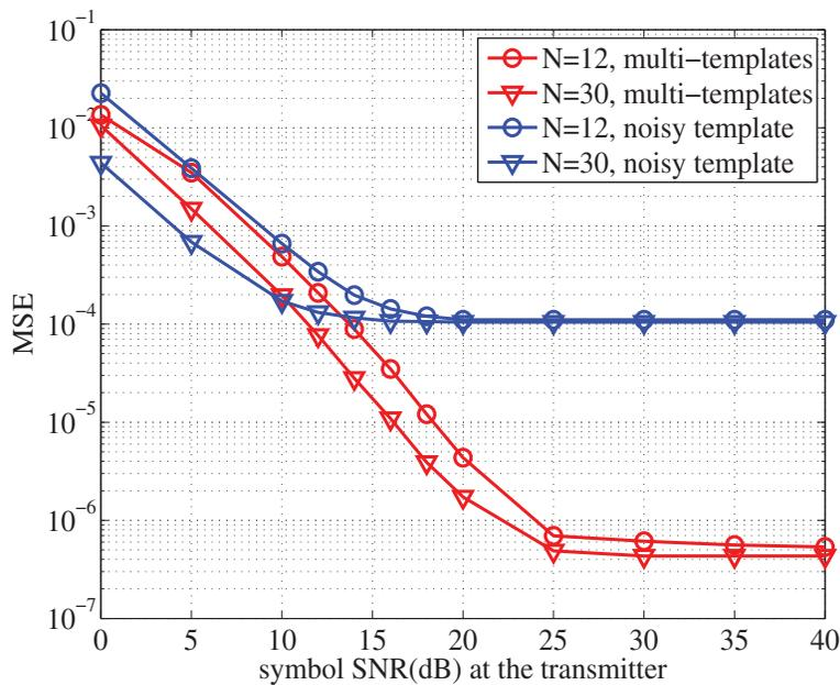
Fig. 2. MSE performance under CM2 with  $d = 4m$  ..
