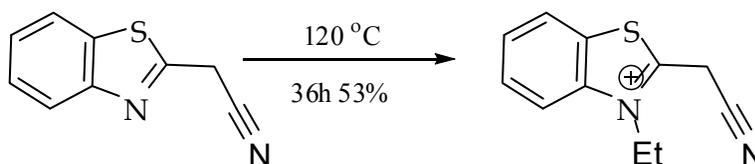
Fig. 12. Synthesis of methylbenzothiazole acetonitrile quaternary salt
