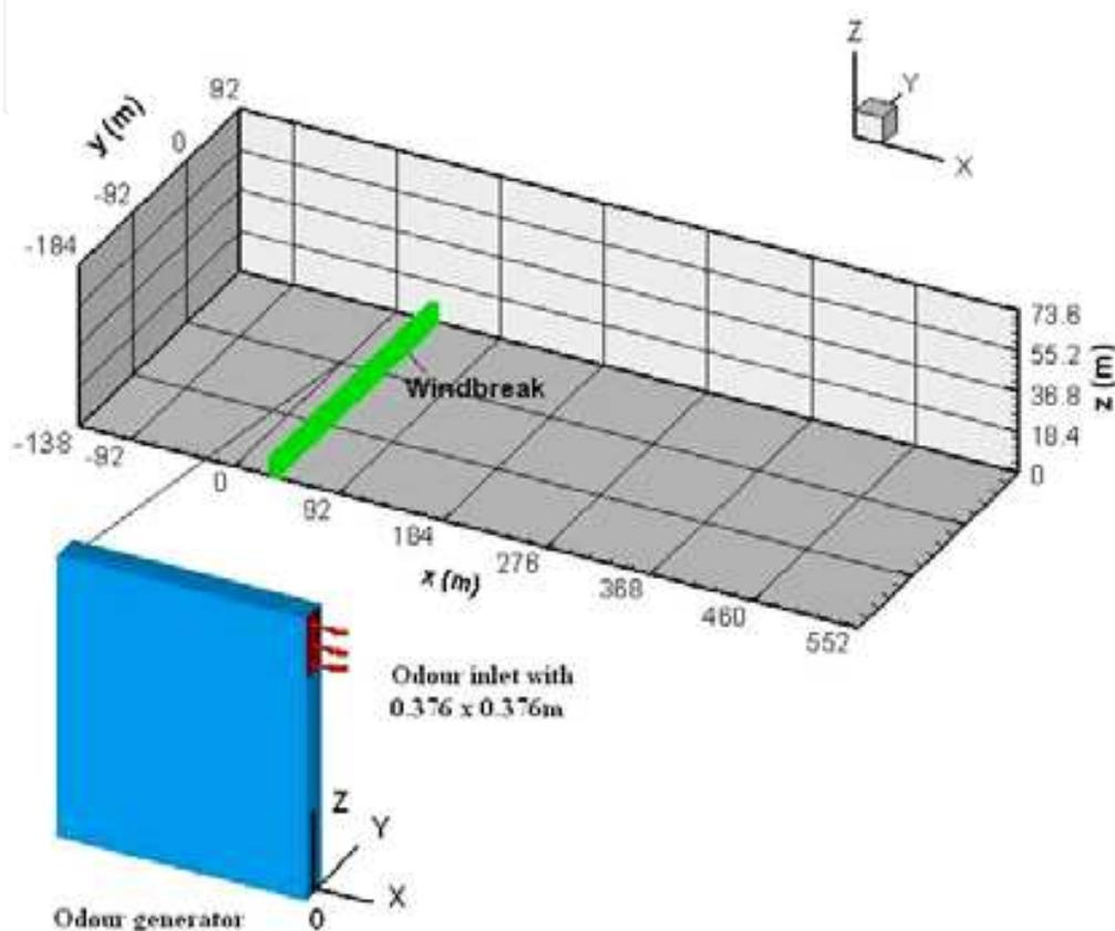
Fig. 4. The computational volume schematics used to predict odour dispersion. In this case, the  $z$  coordinate is magnified 2 times and the windbreak optical porosity is 0.35. The green bar represents the windbreak and the odour emission surface centre of the odour generator is located at  $x = 0$ ,  $y = 0$  and  $z = 1.562$  m
