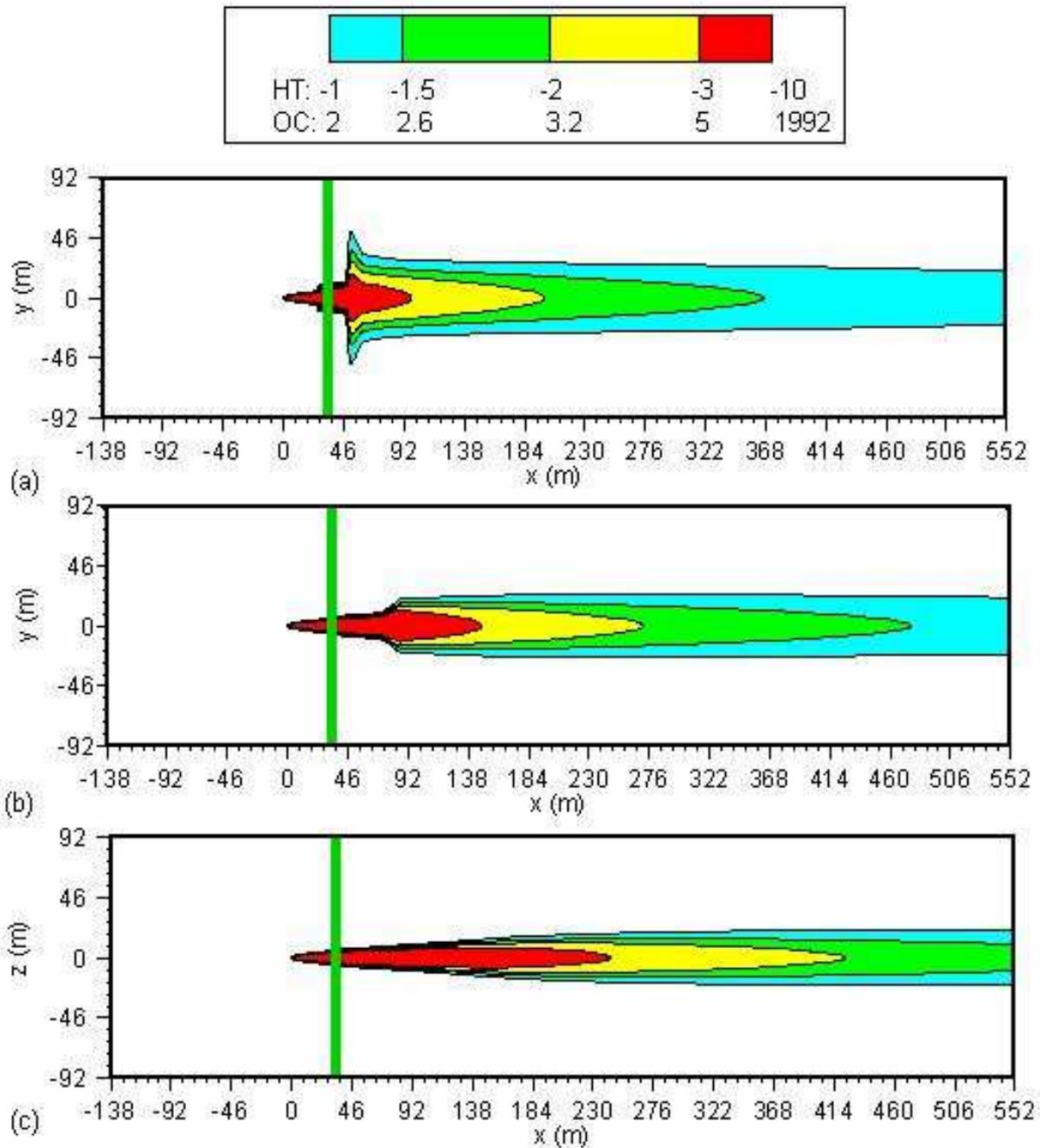
Fig. 10. Contours of the odour plume ( $z = 1.5$  m) for an aerodynamic porosity of (a) 0.2, (b) 0.4 and (c) 0.66, respectively. The green bar is the windbreak and the unit of the odour concentration is  $\text{OU m}^{-3}$  (Lin et al., 2009a)
