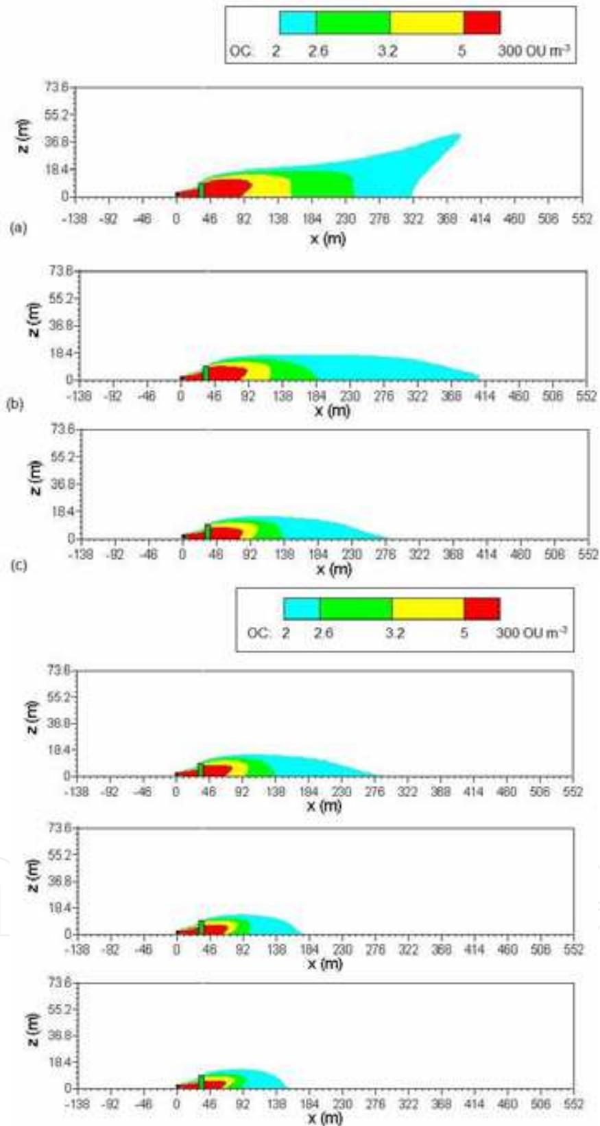
Fig. 12. Effect of wind direction on the odour plume for an horizontal plane at  $z = 1.5$  m, when the wind direction from the positive  $x$ -axis is (a)  $0^\circ$ ; (b)  $15^\circ$ ; (c)  $30^\circ$ , and; (d)  $45^\circ$ . The green bar is the windbreak (Lin et al., 2009b)
