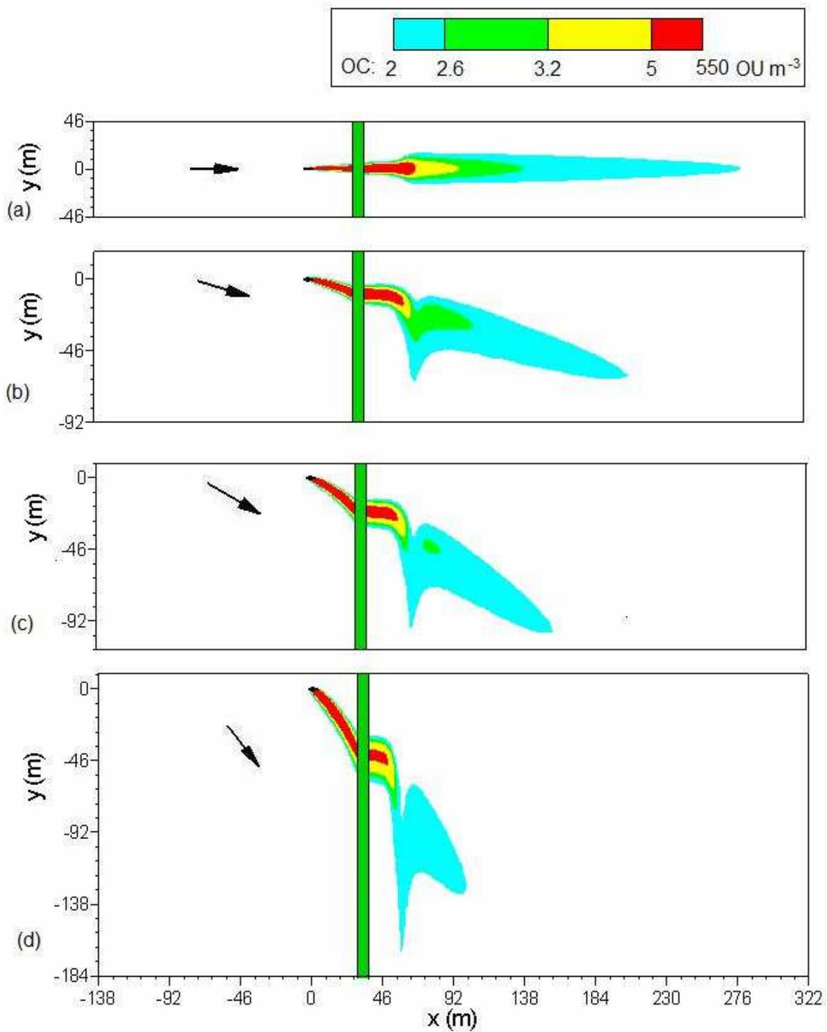
Fig. 11. Effect of wind velocity for: upper) unstable atmosphere for wind velocities of (a) 1.0 m s<sup>-1</sup>; (b) 1.8 m s<sup>-1</sup>, and; (c) 3 m s<sup>-1</sup>; lower) neutral atmosphere for wind velocities (a) 3 m s<sup>-1</sup>; (b) 5.4 m s<sup>-1</sup>, and; (c) 6.4 m s<sup>-1</sup>. The green bar is the windbreak; the odour concentration is in OU m<sup>-3</sup> (Lin et al., 2009b)
