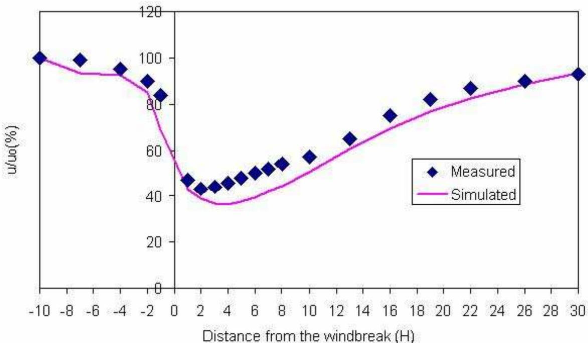
Fig. 8. Comparison of the simulated and measured wind speeds at windbreak half height where  $u$  is the wind speed,  $u_0$  is the undisturbed wind speed, and  $H$  is the height of the windbreak (Lin et al., 2007a). The measured wind speed is taken from Eimern et al. (1964)
