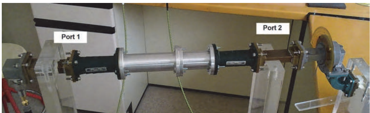
Fig. 8. Waveguide setup for the experimental determination of the rotation angle produced by a chiral material in X-band. A cylindrical sample is located in the circular waveguide and fed through port 1. The transmitted wave is measured in port 2 by a rotating connection, which allows determining the component of the electrical field parallel to the TE_{10} mode of the rectangular wave.
