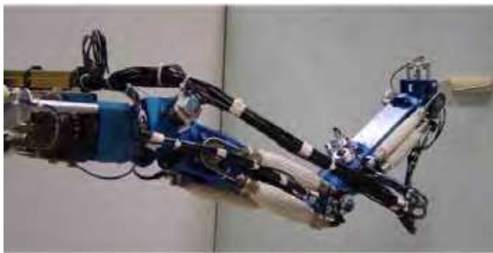
Figure17. Example of a task involving a permanent contact with the environment performed by our 7R anthropomorphic robot-arm actuated by pneumatic McKibben muscle actuators
