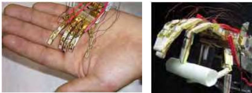
Figure 2. Miniature robot-hand actuated by Nitinol shape memory alloy artificial muscles controlled by heat transfer (from (Maeno & Hino, 2006))
