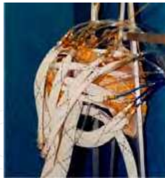
Figure 8. Anthroform Biorobotic Arm project of Washington's BioRobotics Laboratory (Hannaford et al. , 1995) composed of pneumatic McKibben artificial muscles mimicking the shoulder musculature attached to human bones (to our knowledge, no control of the arm has been developed)
