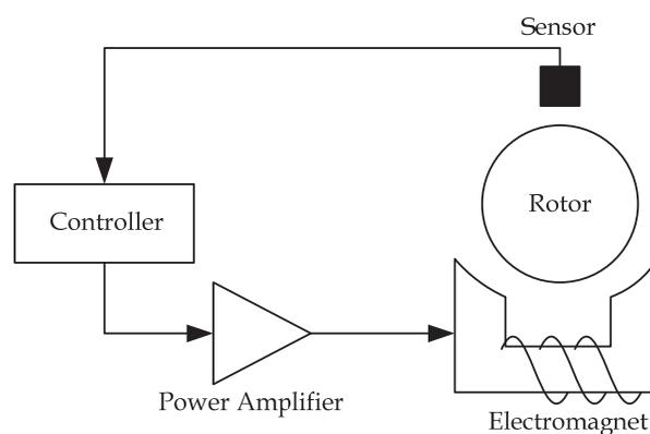
Fig. 8. Diagram of active magnetic suspension system
