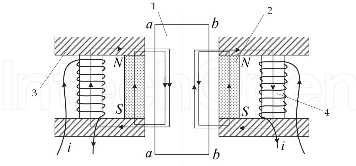
1 rotor, 2 permanent magnets, 3 stator, 4 electromagnet coils.
