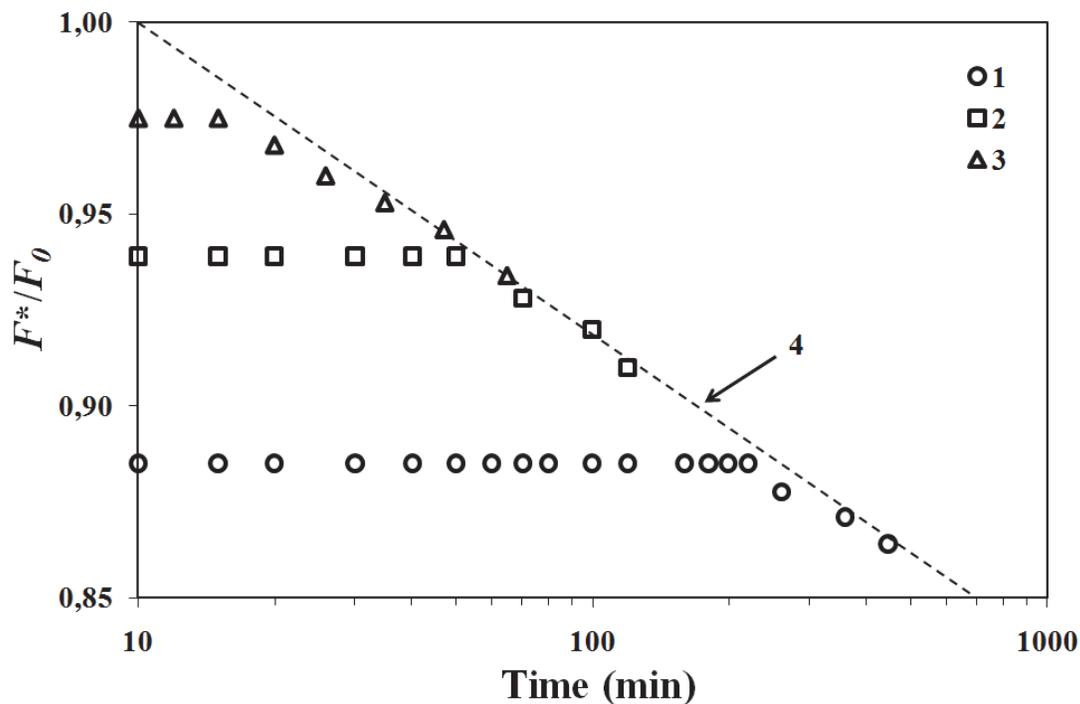
Fig. 3. Normalized magnetic force vs. time for the bipolar magnetization (internal magnetic relaxation) at the different depth of reversal: the initial force  $F_0^* = 230$  mN (dependence 1), 245 mN (2) and 255 mN (3);  $F_0 = 260$  mN. The dashed line 4 is the approximation of data 1 in Fig. 2.
