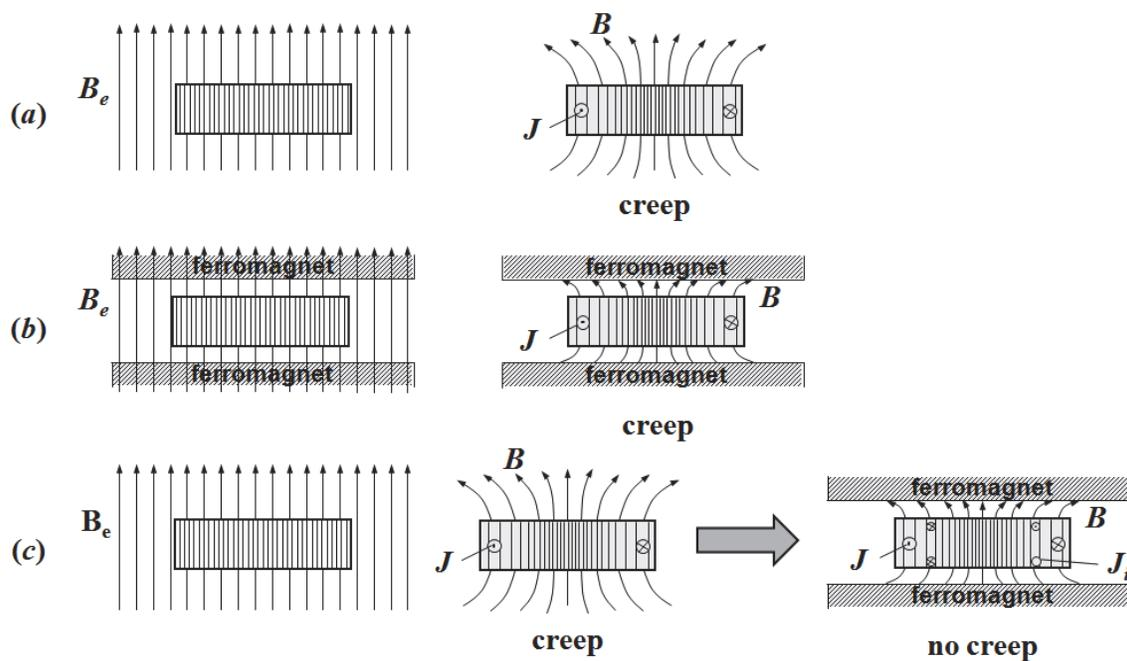
Fig. 6. Magnetizing conditions and relative position of the sample and the ferromagnet in the experiments (a), (b) and (c) (description of the experiments see the text).  $B_e$ , the external magnetic field;  $B$ , the induction of the trapped magnetic flux;  $J$  and  $J_i$ , the density of currents induced in the sample upon trapping of the flux and screening of the ferromagnet field, respectively.
