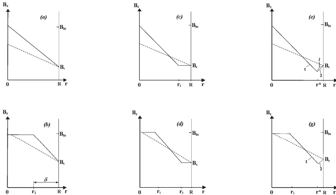
Fig. 1. One-gradient (a)–(d) and two-gradient (e), (g) magnetic flux distributions within the disk at the moment of time  $t'$  (—) and  $t''$  (---); for all distributions  $t'' \gg t'$ . The time  $t'' \geq t_i$  for the distributions (c) and (d);  $t'' \geq t_b$  for the distributions (e) and (g).
