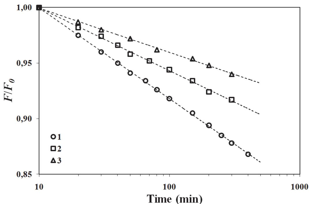
Fig. 2. Normalized magnetic force vs. time for the unipolar magnetization (open magnetic relaxation) at the different penetration depth of critical state: the initial force  $F_0 = 260$  mN (dependence 1), 205 mN (2) and 150 mN (3).
