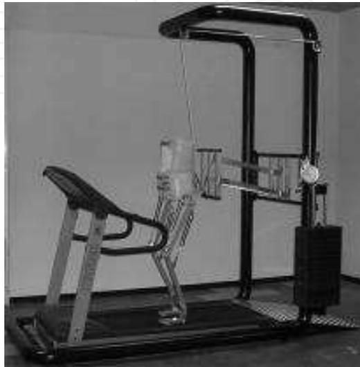
Fig. 5. Realized prototype of the overall rehabilitation system
