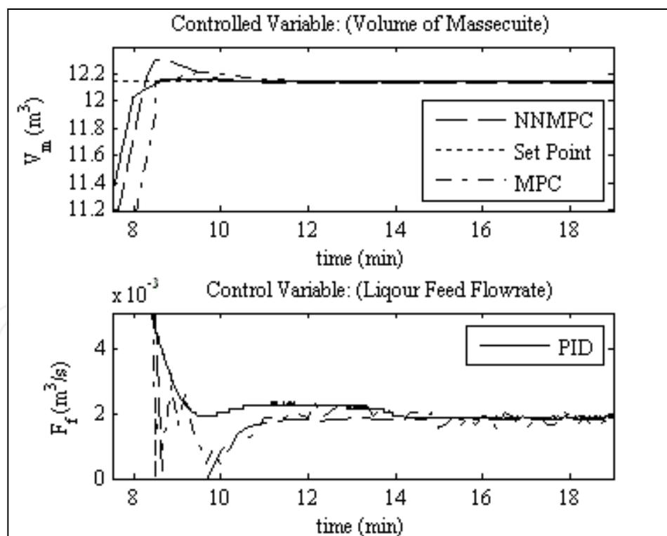
Fig. 4. Controlled (Volume of masecuite) and control variables ( $F_f$ - feed flowrate) over time for the 1<sup>st</sup> control loop.
