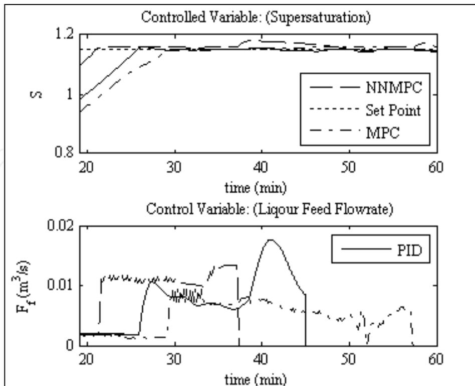
Fig. 5. Controlled (Supersaturation) and control variables ( $F_f$ - feed flowrate) over time for the 2<sup>nd</sup> control loop.
