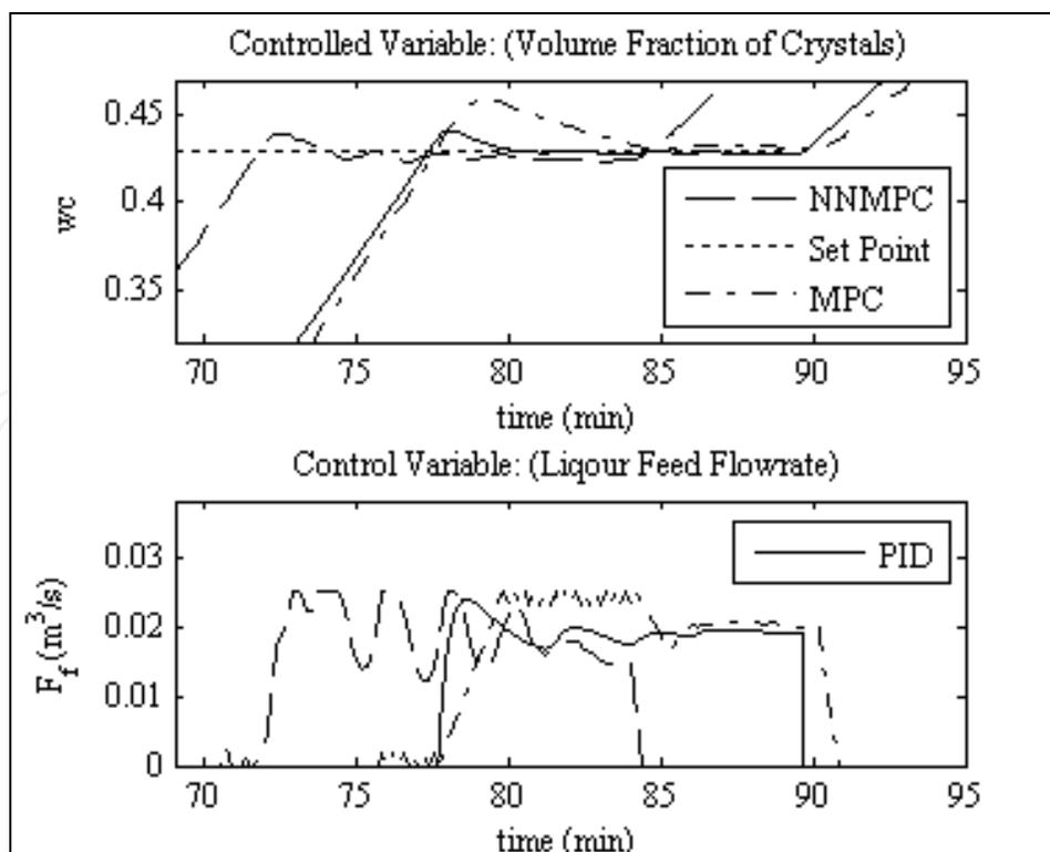
Fig. 6. Controlled (Volume fraction of crystals) and control variables ( $F_f$ - feed flowrate) over time for the 4<sup>th</sup> control loop.
