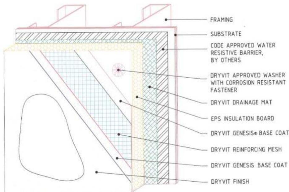
Fig. 5. Typical detail.
