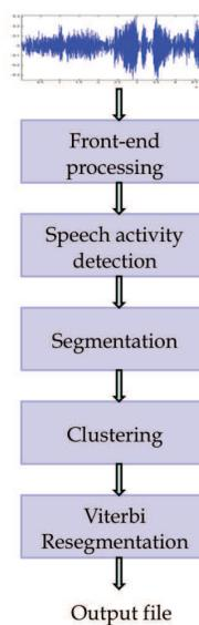
Fig. 1. Flow-chart of a baseline step-by-step algorithm
