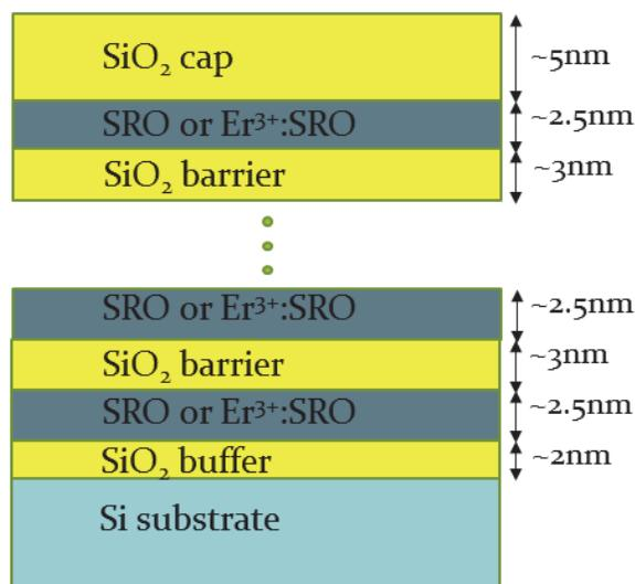
Fig. 2. Cross section of the SRO/SiO<sub>2</sub> and Er<sup>3+</sup>:SRO/SiO<sub>2</sub> superlattice samples deposited by the co-sputtering process
