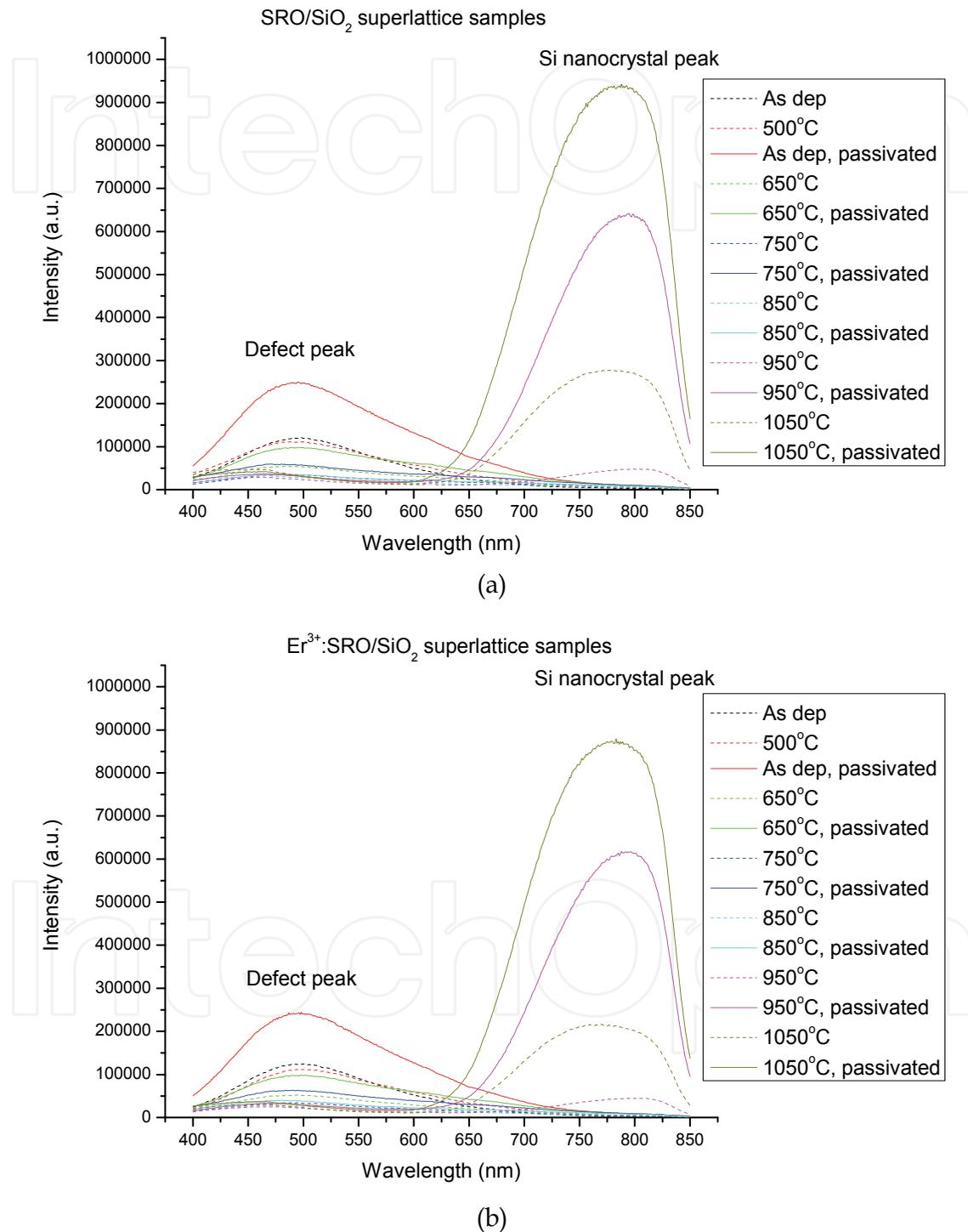
Fig. 6. Visible to near IR PL spectra of (a) the SRO/SiO<sub>2</sub> superlattice samples and (b) the Er<sup>3+</sup>:SRO/SiO<sub>2</sub> superlattice samples at different annealing temperature under the excitation of 290nm
