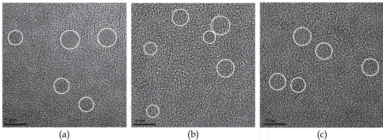
Fig. 3. TEM images of (a) the bulk SRO sample annealed at 850°C, (b) the bulk SRO sample annealed at 950°C, and (c) the SRO/SiO<sub>2</sub> superlattice sample annealed at 950°C
