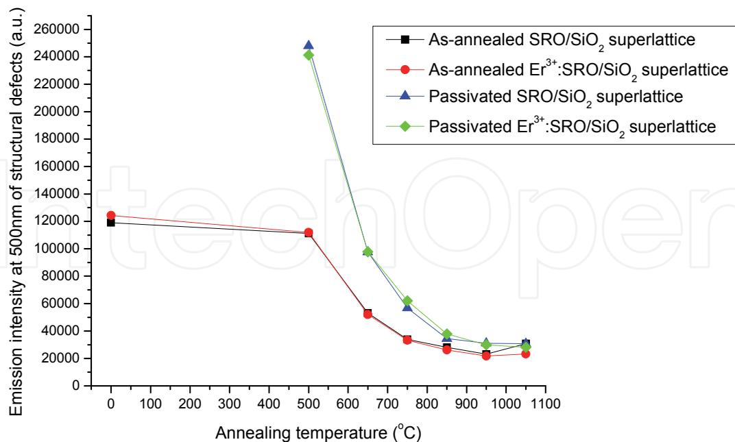
Fig. 7. Evolution of the emission peak at 500nm of the as-annealed and passivated SRO/SiO<sub>2</sub> and Er<sup>3+</sup>:SRO/SiO<sub>2</sub> superlattice samples as a function of the annealing temperature
