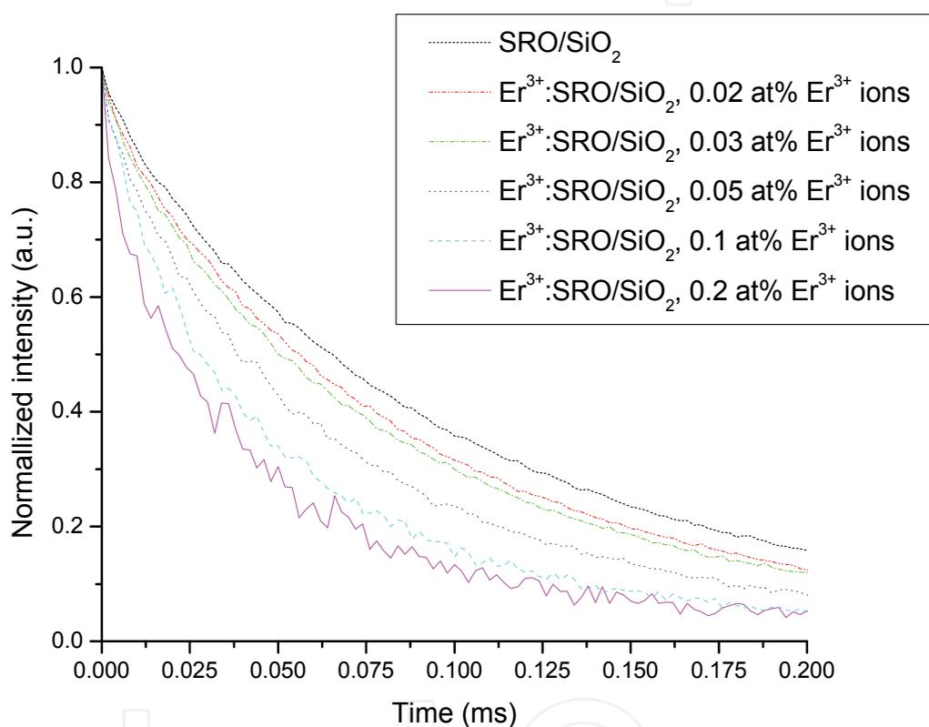
Fig. 11. Normalized room temperature luminescence decay intensity of the exciton recombinations in Si nanocrystals at 800nm of the SRO/SiO<sub>2</sub> and Er<sup>3+</sup>:SRO/SiO<sub>2</sub> superlattice samples with different Er<sup>3+</sup> ion concentration
