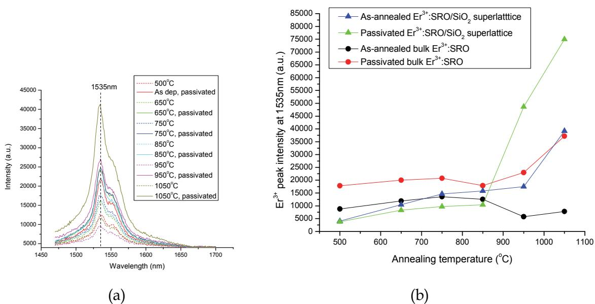
Fig. 8. (a) IR PL spectra at 1470nm-1700nm of the bulk Er<sup>3+</sup>:SRO samples (b) Evolution of the Er<sup>3+</sup> peak intensity at 1535nm as a function of the annealing temperature of the as-annealed and passivated bulk Er<sup>3+</sup>:SRO and Er<sup>3+</sup>:SRO/SiO<sub>2</sub> superlattice samples. The excitation was fixed at 290nm
