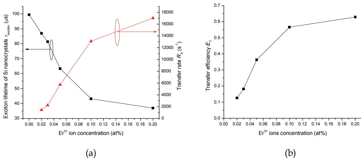
Fig. 13. (a) Exciton lifetime in Si nanocrystals,  $\tau_{exciton}$ , transfer rate,  $R_{tr}$ , and (b) transfer efficiency,  $E_T$ , from the exciton recombinations in Si nanocrystals to  $Er^{3+}$  ions as a function of the  $Er^{3+}$  ion concentration
