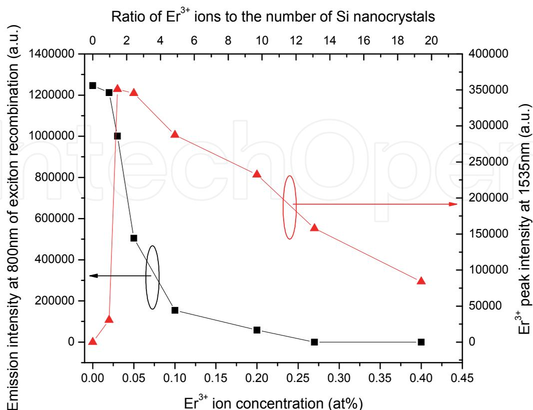
Fig. 10. Variation of the emission intensity at 800nm of the exciton recombinations in Si nanocrystals and the Er<sup>3+</sup> peak intensity at 1535nm as a function of the Er<sup>3+</sup> ion concentration and the ratio of Er<sup>3+</sup> ions to the number of Silicon nanocrystals
