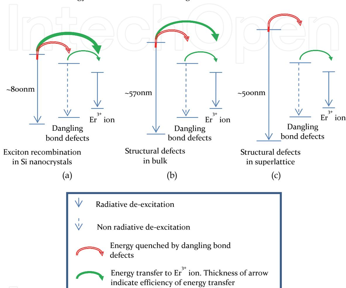
Fig. 9. Different energy transitions and their energy transfer to Er<sup>3+</sup> ions
