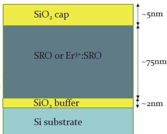
Fig. 1. Cross section of the bulk SRO and Er<sup>3+</sup>:SRO samples deposited by the co-sputtering process
