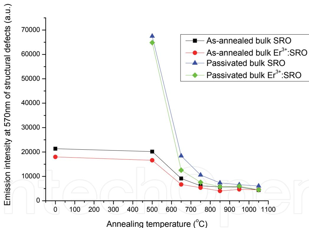
Fig. 5. Evolution of the emission peak at 570nm of the as-annealed and passivated SRO and Er<sup>3+</sup>:SRO samples as a function of the annealing temperature
