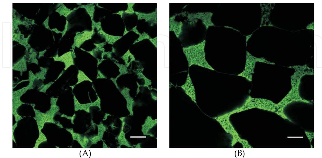
Fig. 4. LSCM images. (A) General aspect of the sandstone porosity. Bar length: 80 μm. (B) Detailed image of pores (communicated channels). Bar length: 40 μm. (C).
