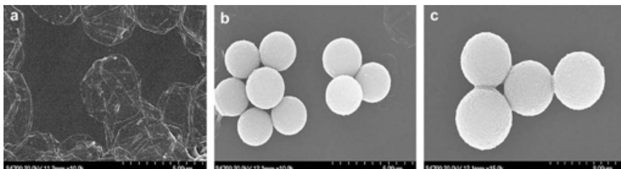
Fig. 10. SEM images of the (ALG/CHI)<sub>5</sub> hollow shells (a) and shells upon incubating the preformed shells in various organic solutions in pure water medium: (b) DCP; (c) SA. Scale bars are 5 mm for a, 5 mm for b and 3 mm for c. (Ding et al., 2009)
