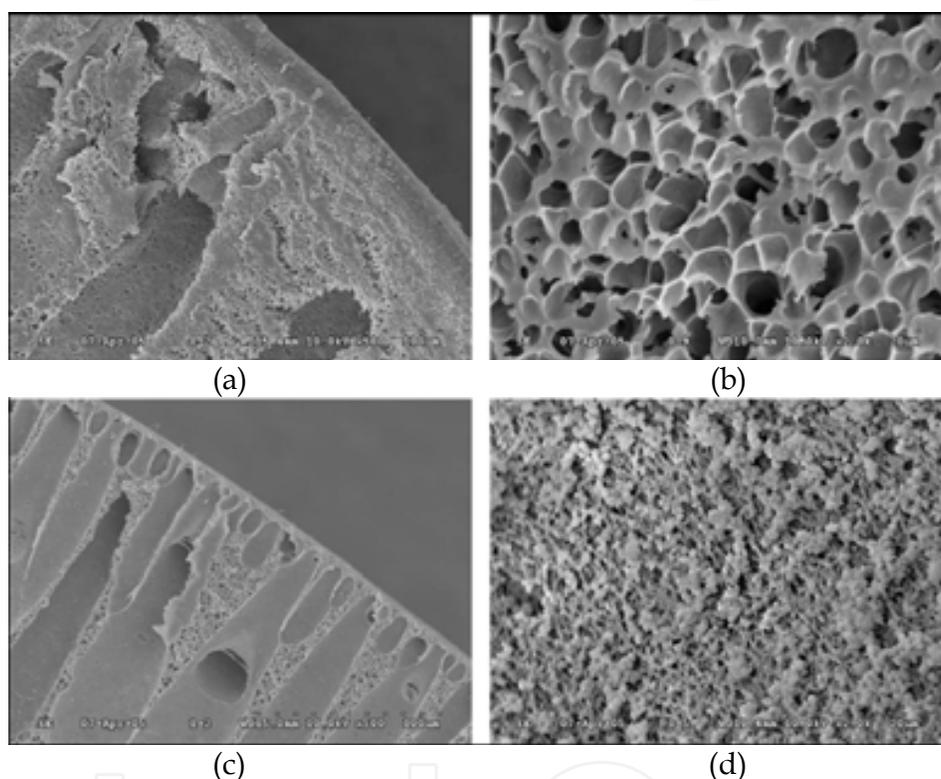
Fig. 9. SEM micrographs of cross-sections of CA and CA-triolein adsorbents. (a) CA adsorbent ( $\times 500$ ), (b) CA adsorbent ( $\times 2000$ ), (c) CA-triolein adsorbent containing 2.0% (w/w) triolein ( $\times 500$ ), and (d) CA-triolein adsorbent containing 2.0% (w/w) triolein ( $\times 2000$ ). (Liu et al., 2007)
