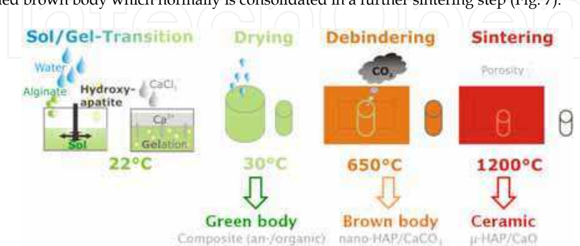
Fig. 7. Sketch of ceramic processing using sol-gel-technique of ionotropic gelation of alginate slurries with ceramic powders
