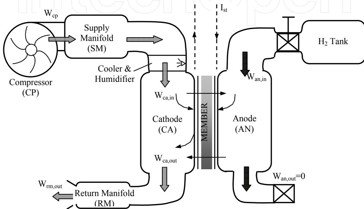
Fig. 5. Simplified fuel cell reactant supply system
