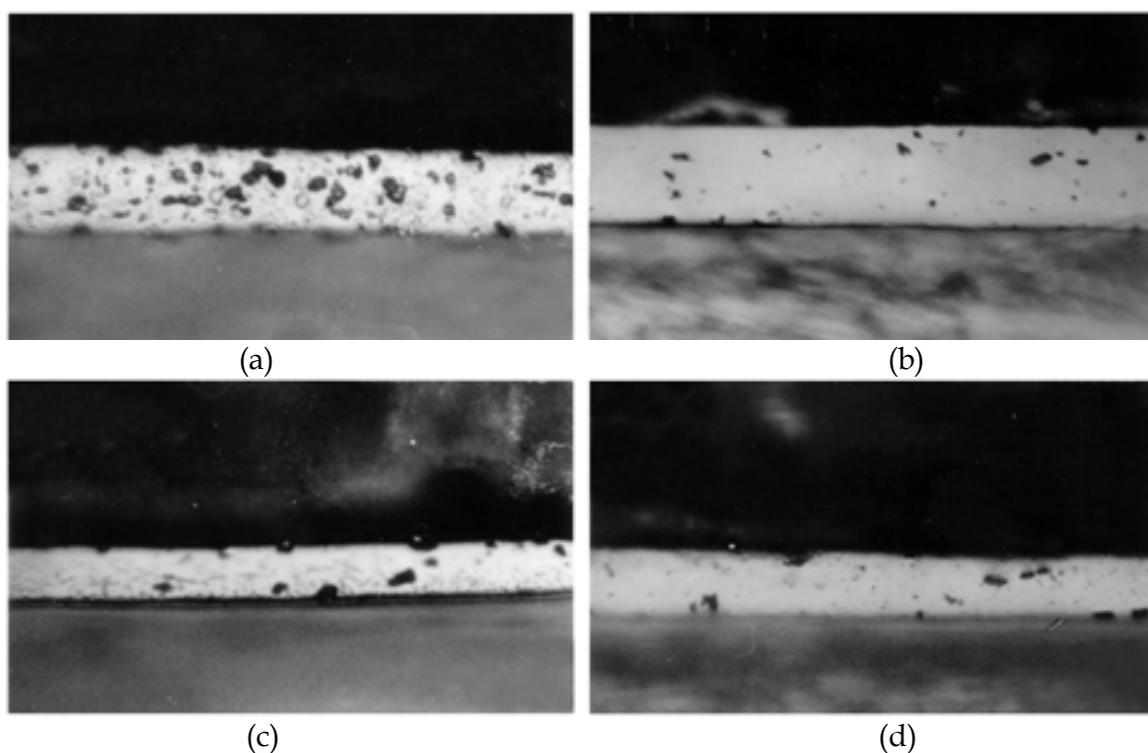
Fig. 6. Photomicrographs of the cross sections of nickel–alumina composite coatings electrodeposited with an average pulse current density of 5 A dm<sup>2</sup> and at various pulse duty cycles and frequencies. (a)- 20% duty cycle and 50 Hz frequency, (b)- 80% duty cycle and 50 Hz frequency, (c)- 60% duty cycle and 20 Hz frequency, (d)- 60% duty cycle and 80 Hz frequency (Bahrololoom & Sani, 2005). (Reprint with the permission from Elsevier Limited)
