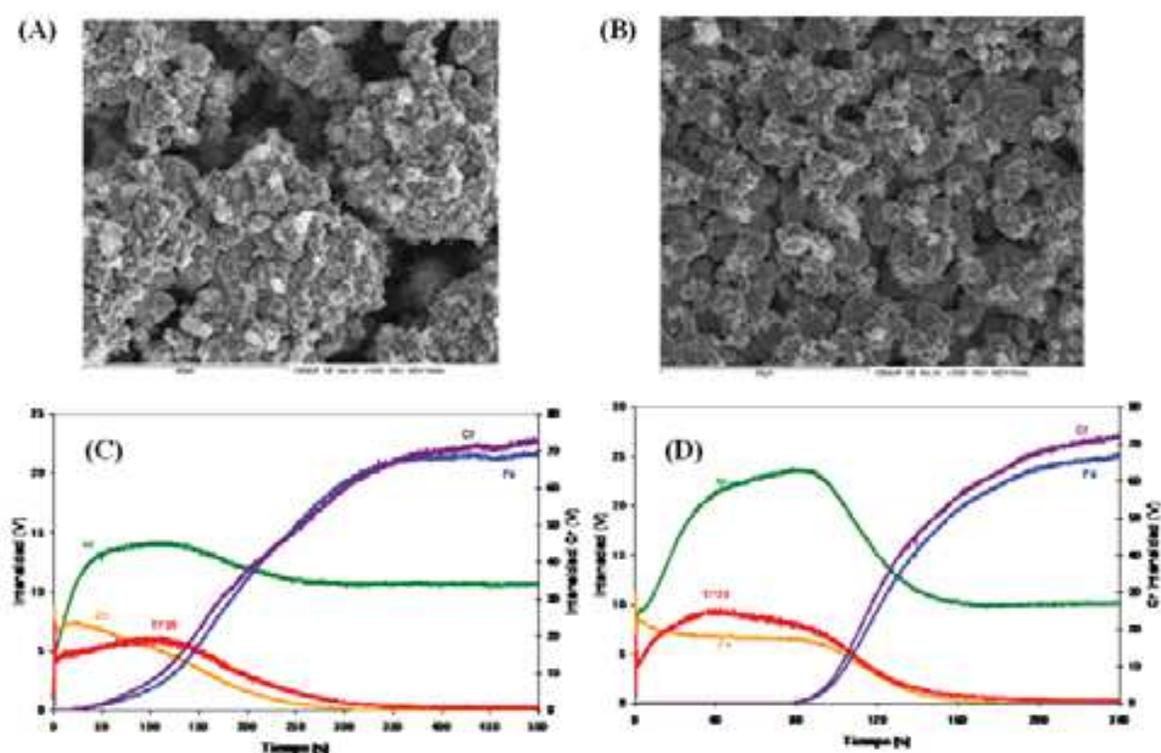
Fig. 9. Characterization of Ni-Zn-TiO<sub>2</sub> nanocomposite films deposited onto steel A & B) SEM images in sulphate and chloride baths, respectively C & D). Qualitative depth profiles obtained by GD-OES (600 Pa, 30 W) in sulphate and chloride baths, respectively (Fernández et al., 2010).
