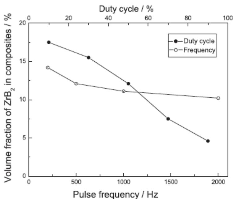
Fig. 5. Effect of the pulse frequency with 50% duty cycle and the duty cycle with 500 Hz frequency on the volume fraction of embedded ZrB<sub>2</sub> particles at an average current density of 5 A dm<sup>-2</sup> (Guo et al., 2006). (Reprint with the permission from Institute of Metal Research)
