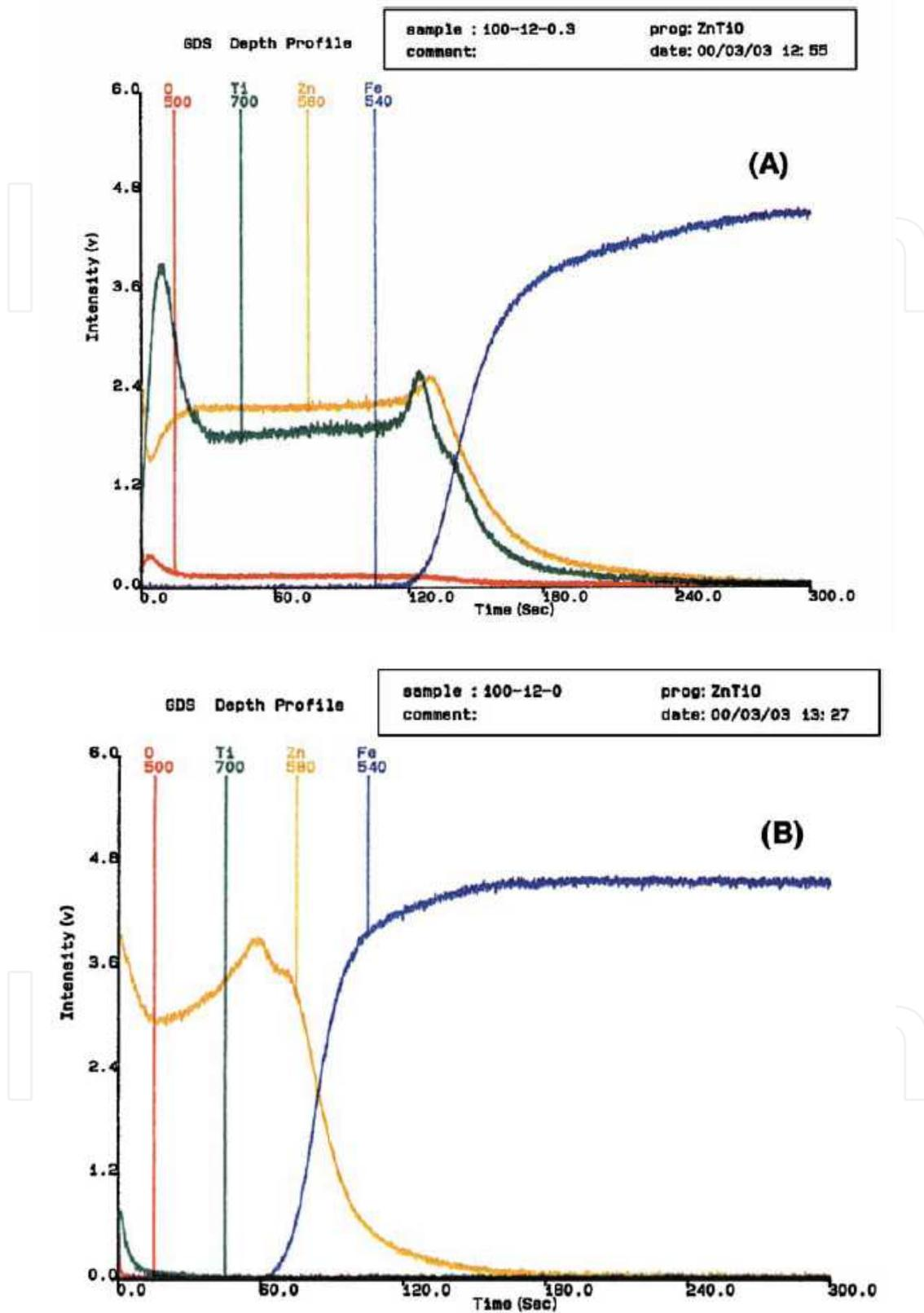
Fig. 8. GD-OES depth profiles for the  $\text{TiO}_2\text{-Zn}$  nanocomposite films prepared at  $I_d = 12 \text{ A dm}^{-2}$ . A)  $\text{TiO}_2\text{-Zn}(0.3,100)/\text{Steel}$ ; B)  $\text{TiO}_2\text{-Zn}(0,100)/\text{Steel}$  (Deguchi et al., 2001). (Reprint with the permission from Springer)
