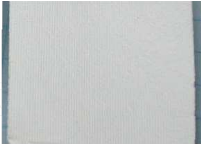
Fig. 6. Wavy membrane prepared from HAp/Col flexible membrane.
