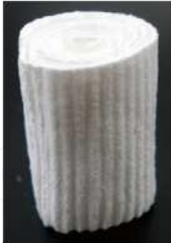
Fig. 8. Unidirectional porous HAp/Col bone-like nanocomposite.
