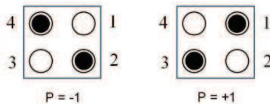
Fig. 1. QCA cell and its ground states
