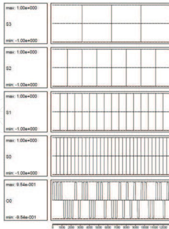
Fig. 13. Simulation Result of Logic-Based S-Box
