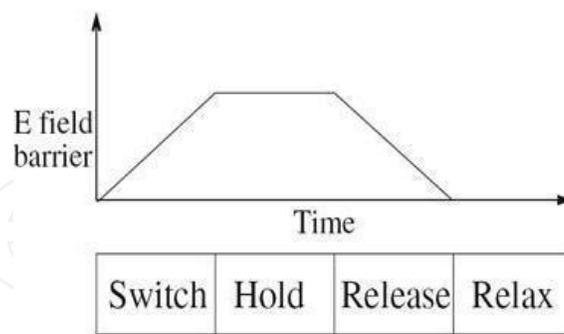
Fig. 5. Barrier height in four phases of clock
