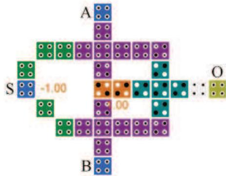
Fig. 9. QCA layout of 2 to 1 multiplexer
