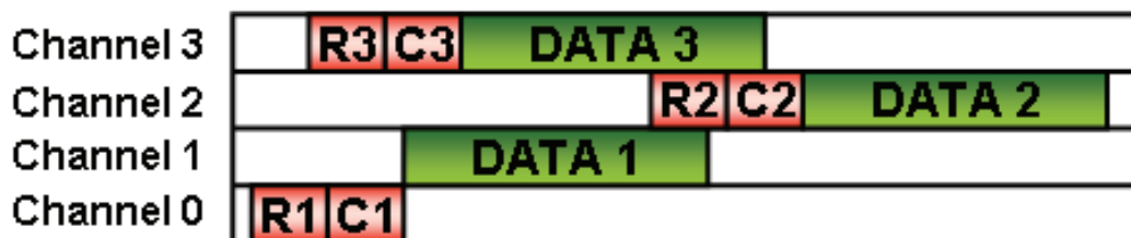
Fig. 5. Common Hopping Approach (figure inspired from [mo07])
