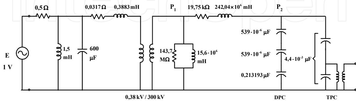
Fig. 23. Electric model of the test setup, with series  $0.5\Omega$  resistance, shunt  $1.5\text{mH}$  and  $600\mu\text{F}$  capacitance for passive reactive compensation applied at the low voltage side of the step-up transformer.
