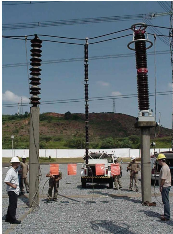
Fig. 1. Capacitive voltage divider (CVD) - installation for measurements in a 345kV substation.
