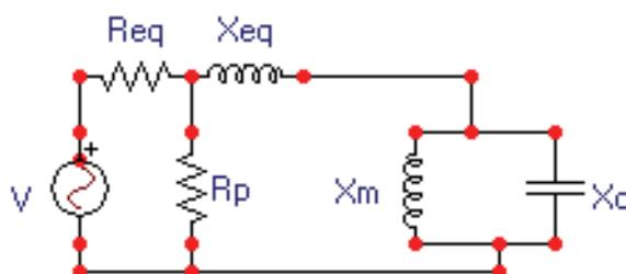
Fig. 6. Test circuit electrical model.
