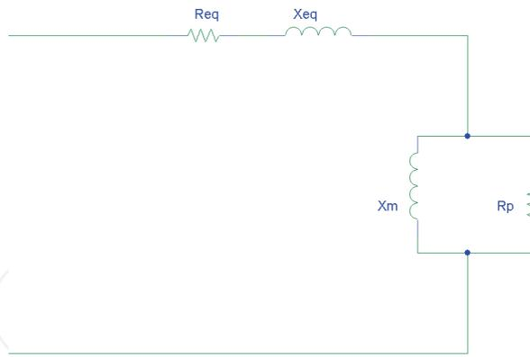
Fig. 3. Equivalent circuit of high voltage transformer where:  $R_{eq}$  – equivalent resistance,  $X_{eq}$  – equivalent leakage reactance,  $X_m$  – magnetizing reactance,  $R_p$  – equivalent no-load loss resistance.
