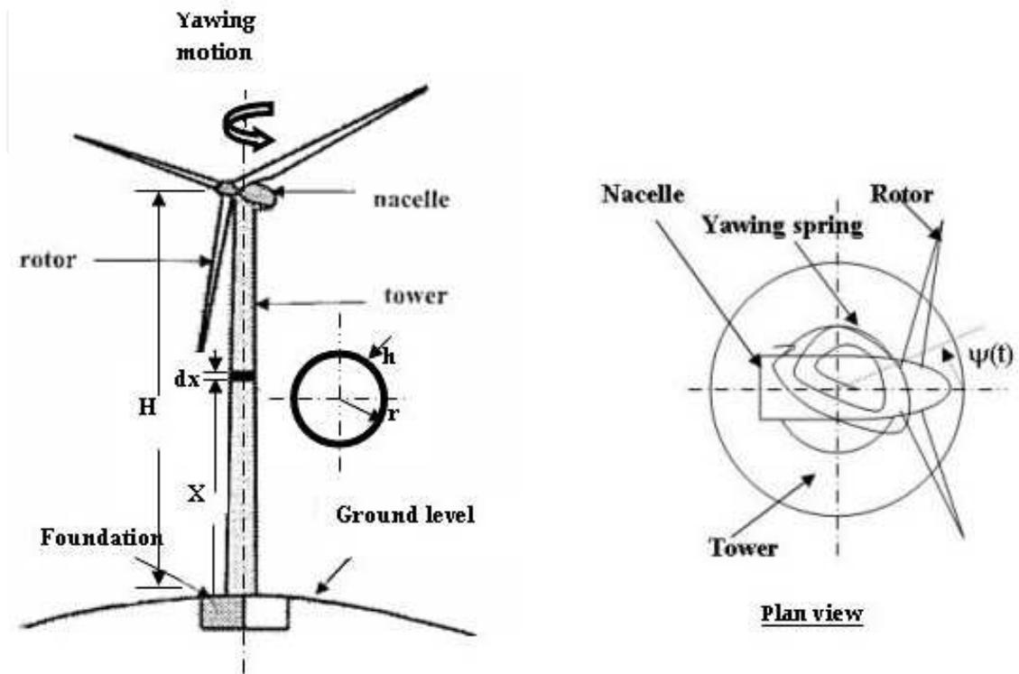
Fig. 5. Horizontal-axis wind turbine in free yawing motion
