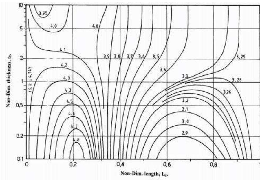
Fig. 11. Second-mode frequency of a teetered blade
