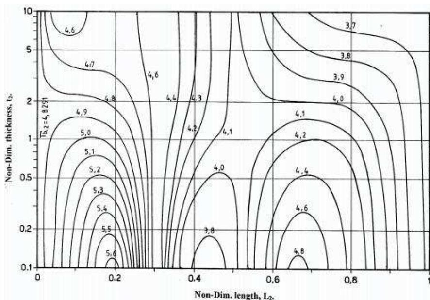
Fig. 10. Second-mode flapping frequency of a hingeless blade
