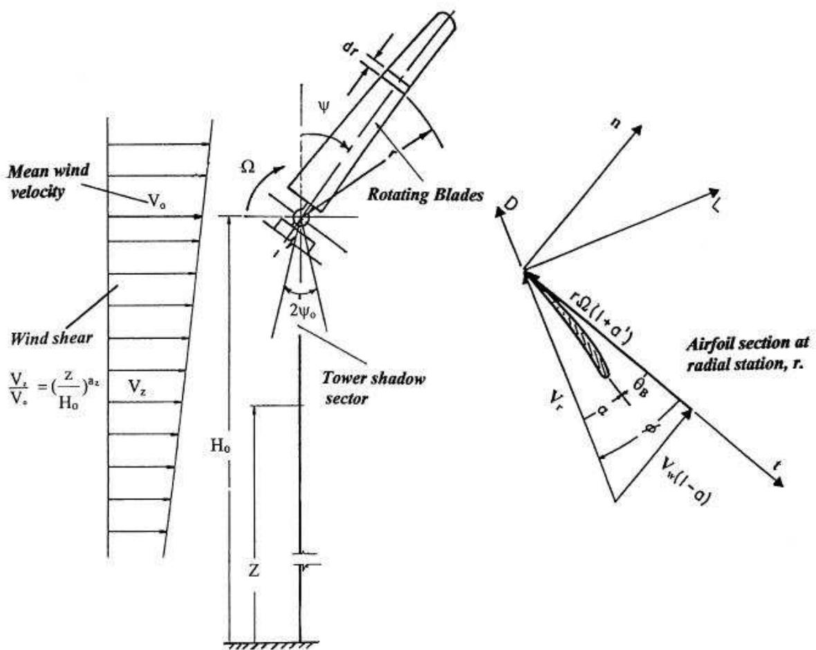
Fig. 3. Wind rotor geometry and velocity components
