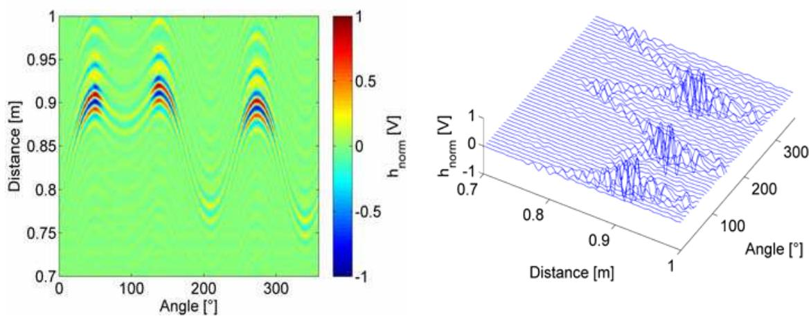
Fig. 5. Measured radargram of object o3 (left) and every 8<sup>th</sup> pulse of same Radar data (right)
