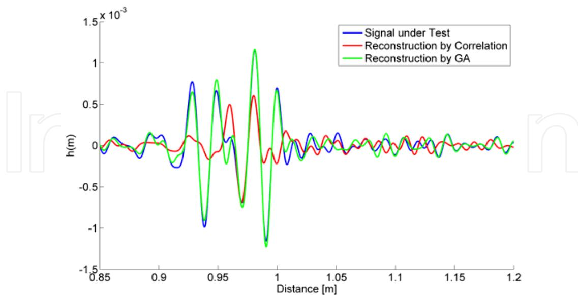
Fig. 13. Reconstruction of a signal under test with both wavefront detection algorithms
