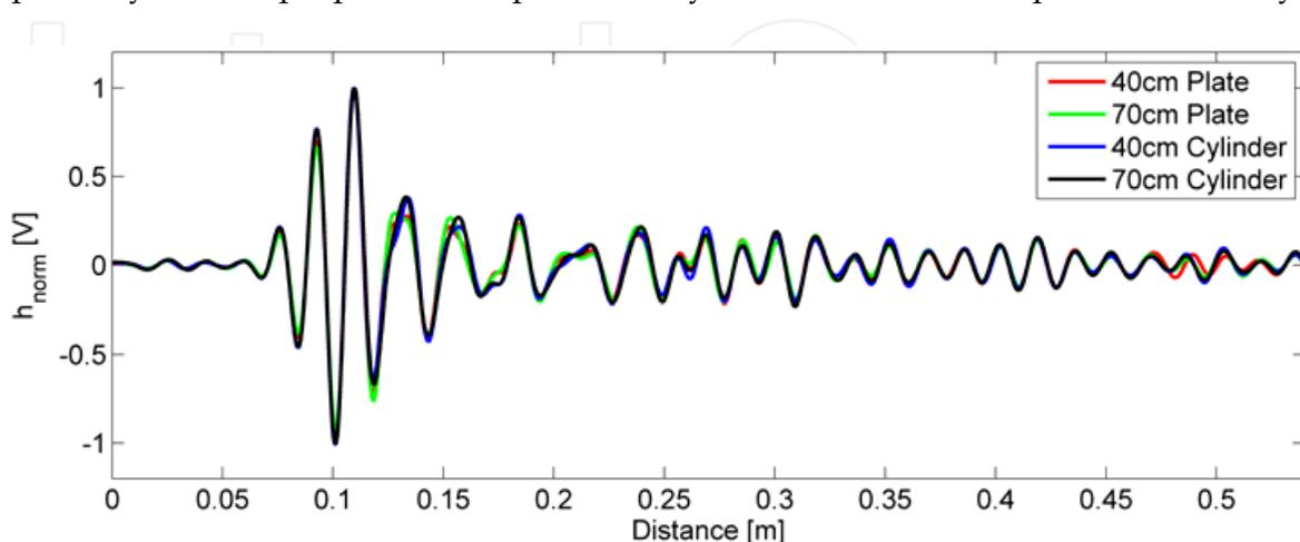
Fig. 7. A set of reference pulses taken at different distances against a plate and cylinder with normalised amplitude and delay
