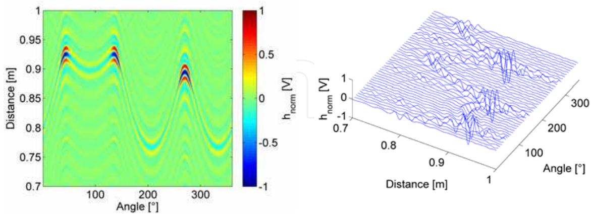
Fig. 4. Radargram of simulated object o3 (left) and every 8<sup>th</sup> pulse of same Radar data (right)
