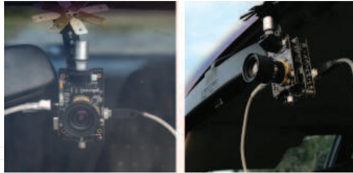
Fig. 3. Camera used to collect data for training and testing. The camera is powered by USB cable connected to a laptop PC.
