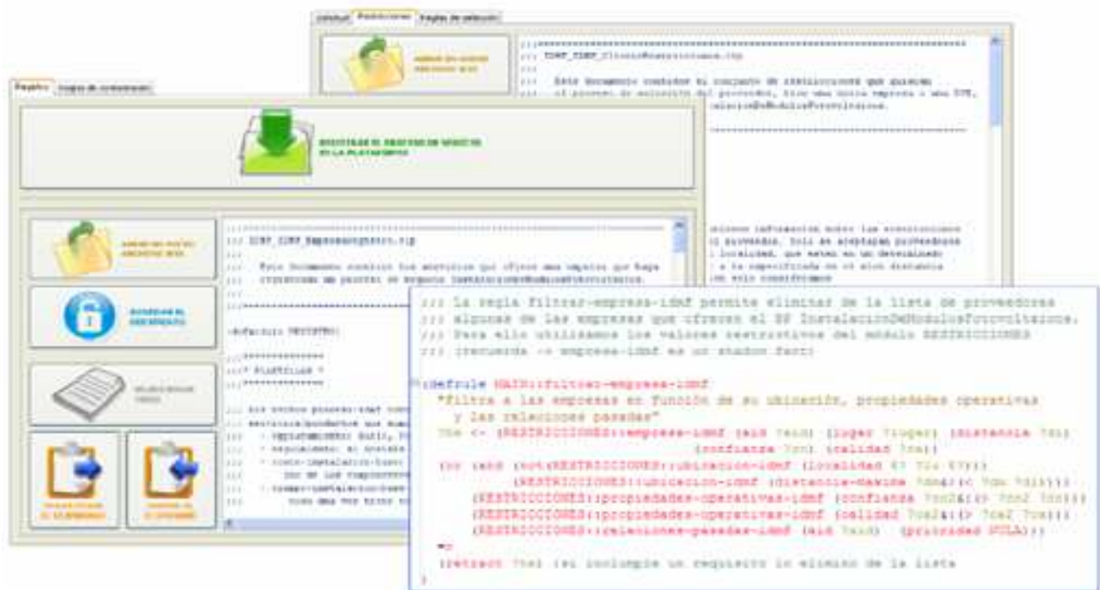
Fig. 12. Example both of a Jess rule and of the GUIs where the decision modules of agents can be modified
