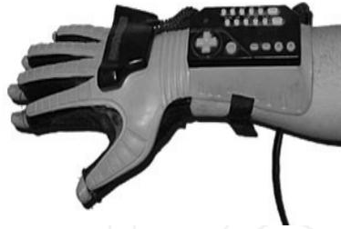
Fig. 5. An instrumented glove (Nintendo power glove)
