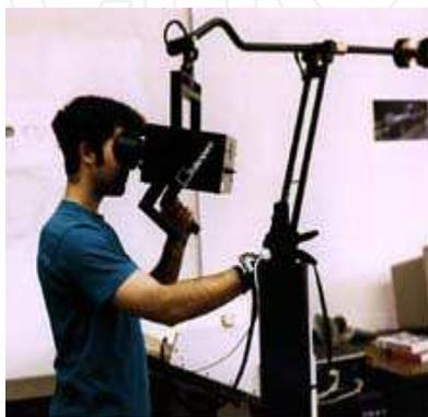
Fig. 2. A Binocular Omni-Orientation Monitor (BOOM)
