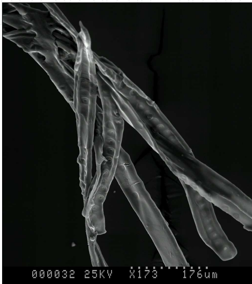
Fig. 7. Treated pine sapwood whose tracheids are easily manually disjoined. Softening and darkening are strongly related and both phenomena imply a lignin modification.
