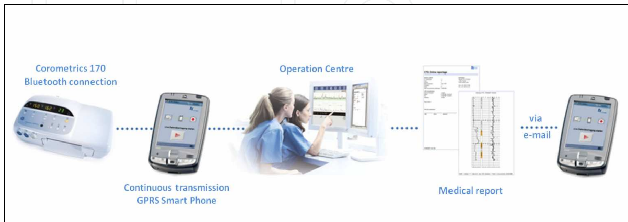
Fig. 1. Organization of the new TOCOMAT network for Telecardiotocography.
