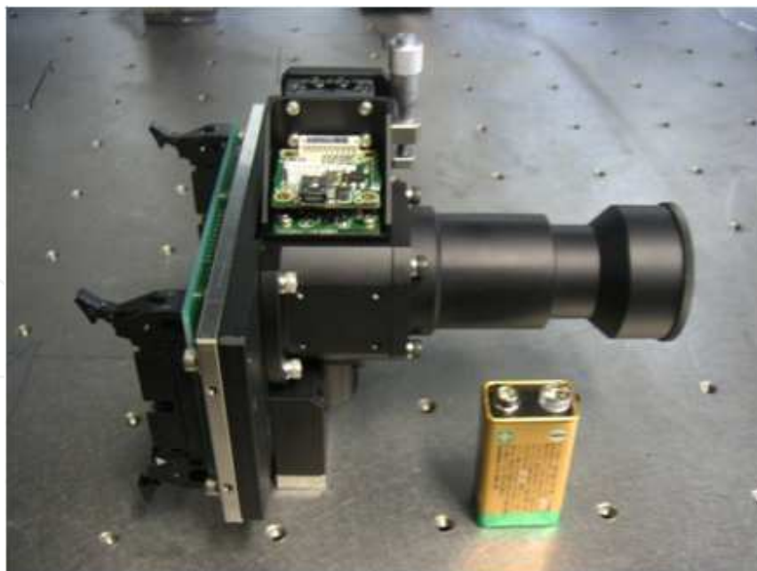
Fig. 5. Optical part of the compact laser communication transceiver
