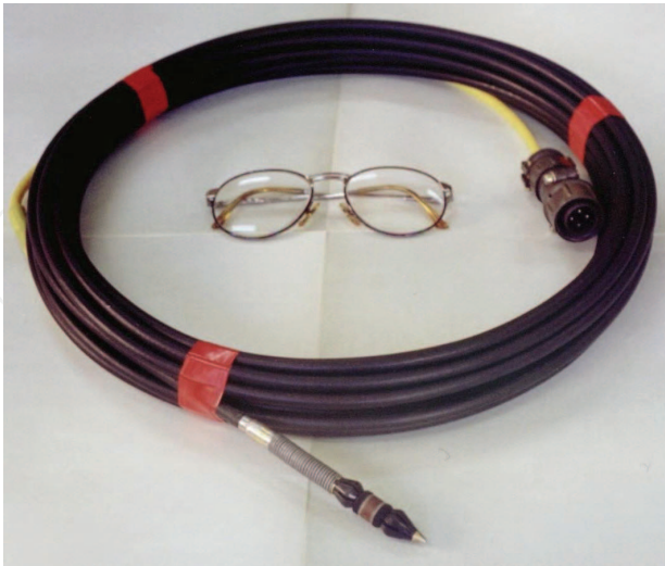
Fig. 14. EC probes for heat exchanger tube inspection.
